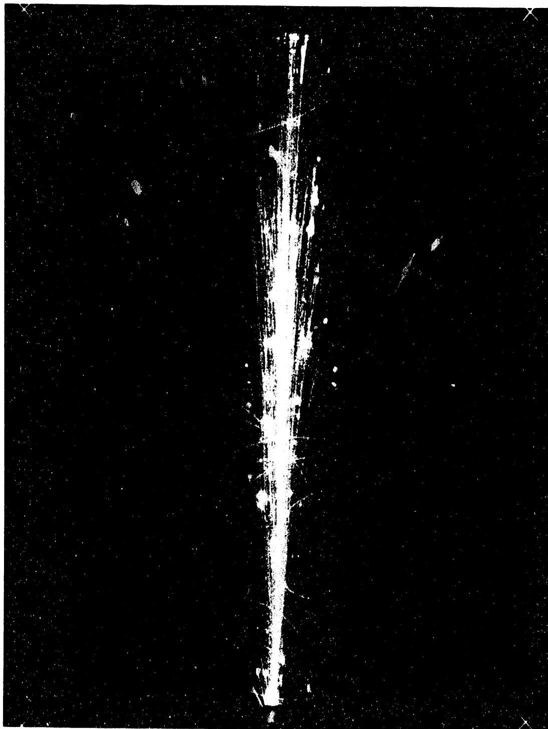
Figure 2.4: Film image of a ^{32}\text{S} + ^{32}\text{S} collision at 200 GeV/nucleon incident energy.
