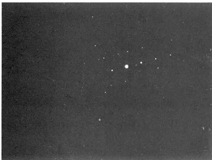
Figure 38b. Diffraction pattern of above twin boundary.
