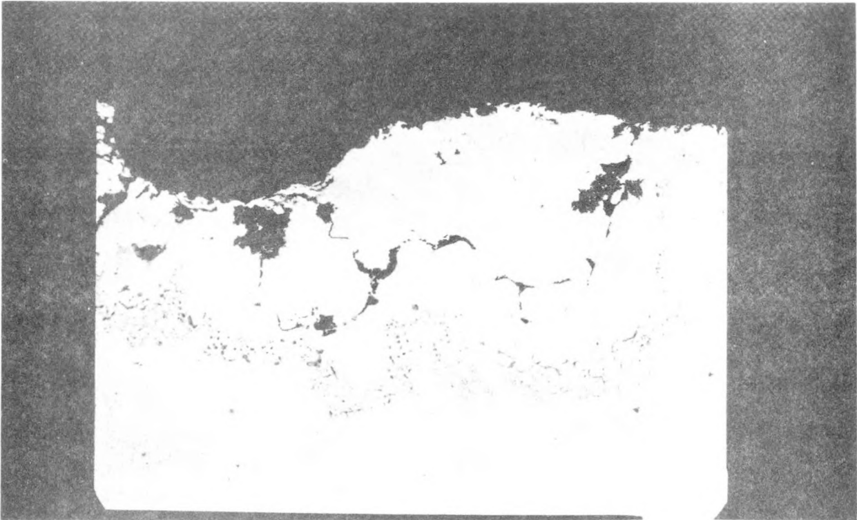
Inconel 600 250X Oxidation and Sulfidation
