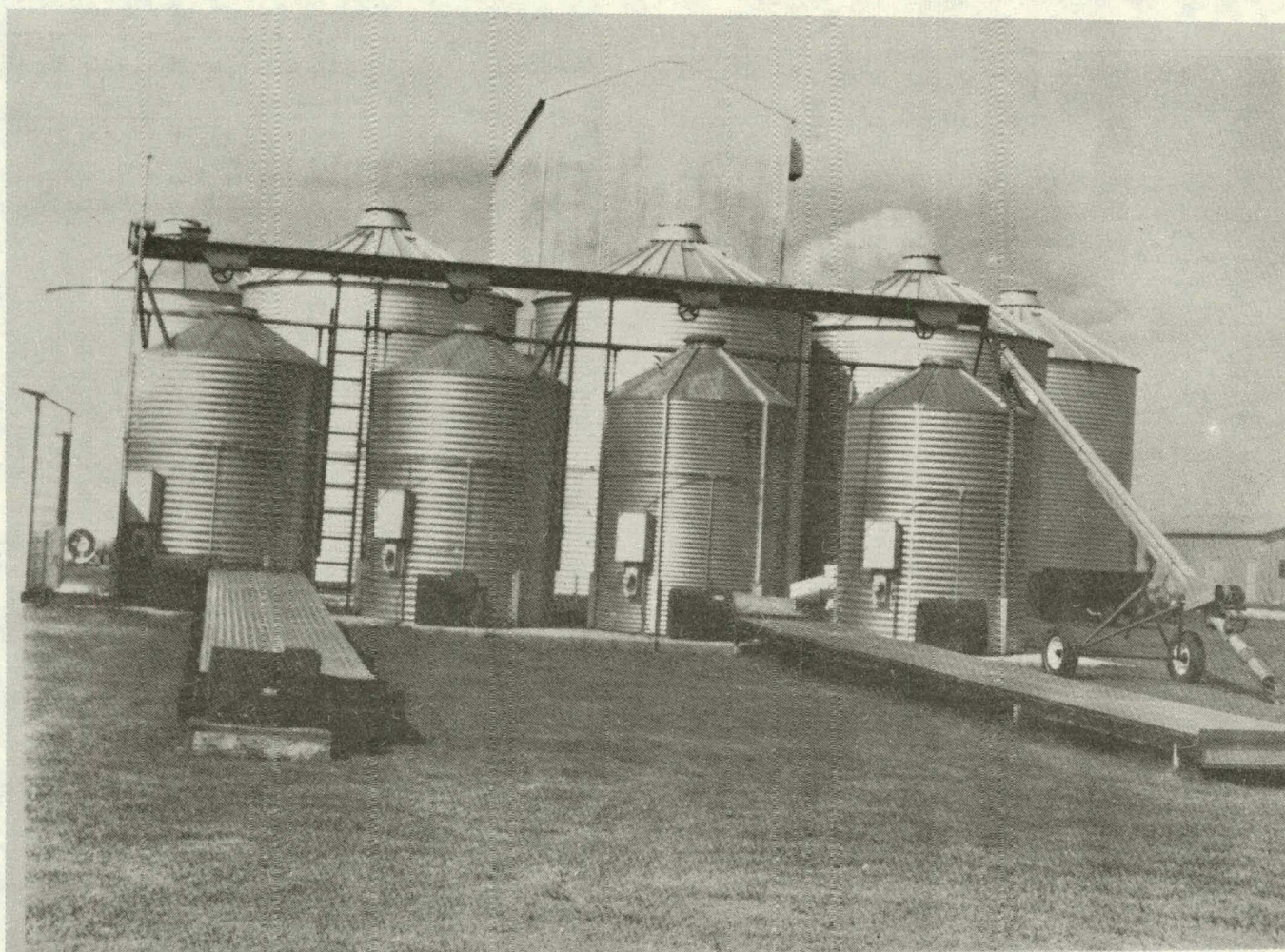
Figure 1. Solar rice drying test installation in 1975. Shown from left to right: Bin 1, with a solar collector and no stirring auger; Bin 2, without a solar collector or stirring auger; Bin 3, with both a solar collector and a stirring auger; Bin 4, with a stirring auger but no solar collector.
