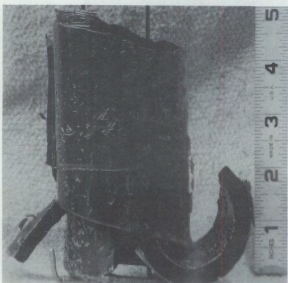
FIGURE 4.5. Appearance of Water-Reacted Outer Element on Holder Following Run 9
