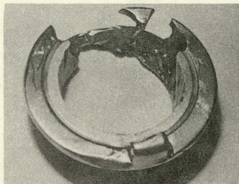
Figure 14-7. Erosion Damage to Stainless-Steel Plug and Seat After Service in a Slurry-Recirculation Valve
