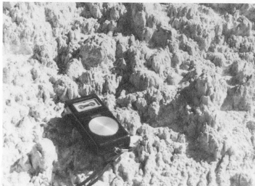
Figure 2-4. Photographs of Drying Crust on Slopes of Gypsum Stack
