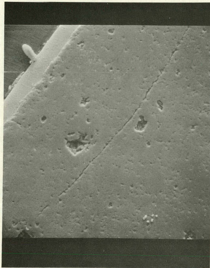
Fig. 47. Scanning Electron Micrograph of Crack Indicated in Fig. 46. ANL Neg. No. 306-77-488.
