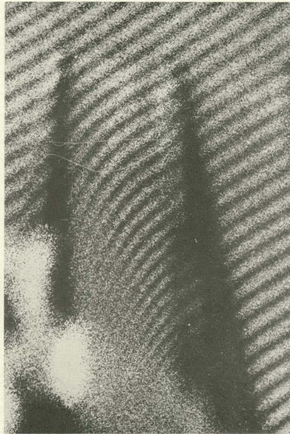
Fig. 21. Picture of Blade Loaded in Bending in Its Own Plane. Improved resolution. ANL Neg. No. 306-77-491.
