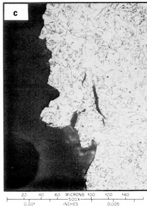
Fig. 5.12. Metallographic examination of the crack tip region of PCCy specimen V8W69. This specimen was tested at -73^{\circ}\text{C} and exhibited a fracture toughness of 70 \text{ MN}\cdot\text{m}^{-3/2} . The crack tip resides in the refined region of the weld metal microstructure as shown in (a) at the magnification of 25\times . The microstructure in this region is shown in (b). Original reduced 15%.
