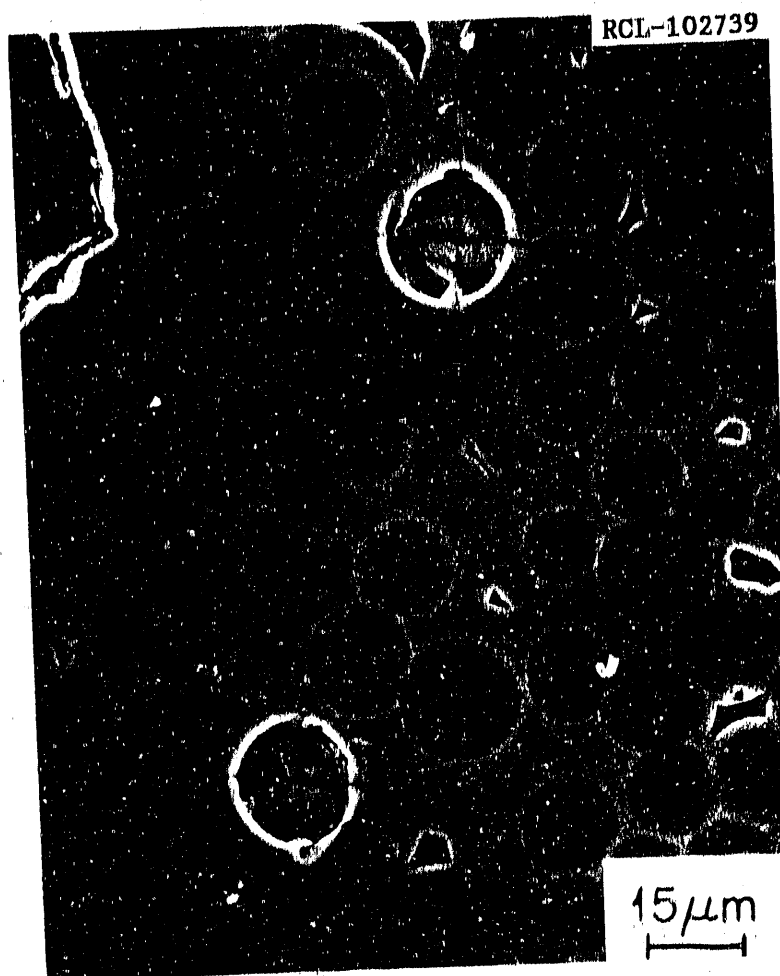
Figure 10.10. SEM micrograph showing indented silicon-coated Nicalon fibers.
