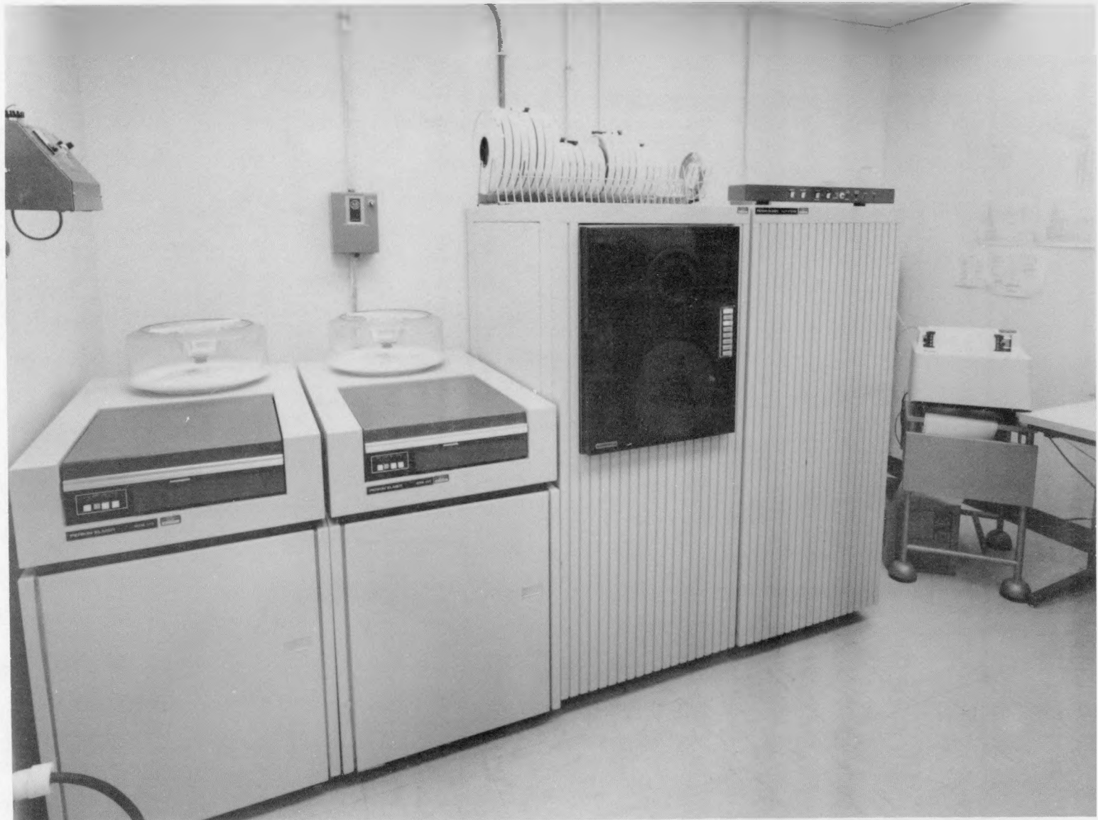
FIGURE 2.51. PE3220 Computer System Used to Control and Receive Data for the ASEM System. Neg 8102282-3
