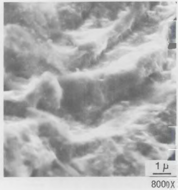
FIGURE 16. SEM Micrographs of \text{UO}_2 Surfaces After 11 Days at 150^\circ\text{C} in \text{NaHCO}_3 (0.03 M) Containing 200 ppm Dissolved Oxygen
