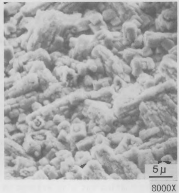
FIGURE 14. SEM Micrographs of \text{UO}_2 Surfaces After 60 Days at 150^\circ\text{C} in Deionized Water Containing 200 ppm Dissolved Oxygen
