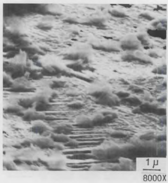
FIGURE 24. SEM Micrographs of \text{UO}_2 Surfaces After 30 Days at 150^\circ\text{C} in WIPP "B" Brine Solution Containing 200 ppm Dissolved Oxygen
