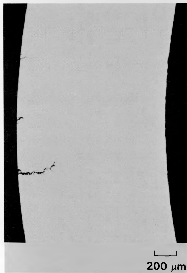
FIGURE 3.28. Optical Micrographs Showing Axial IGSCC at the Apex of U-Bend Specimen 1049 (R2 C27)
