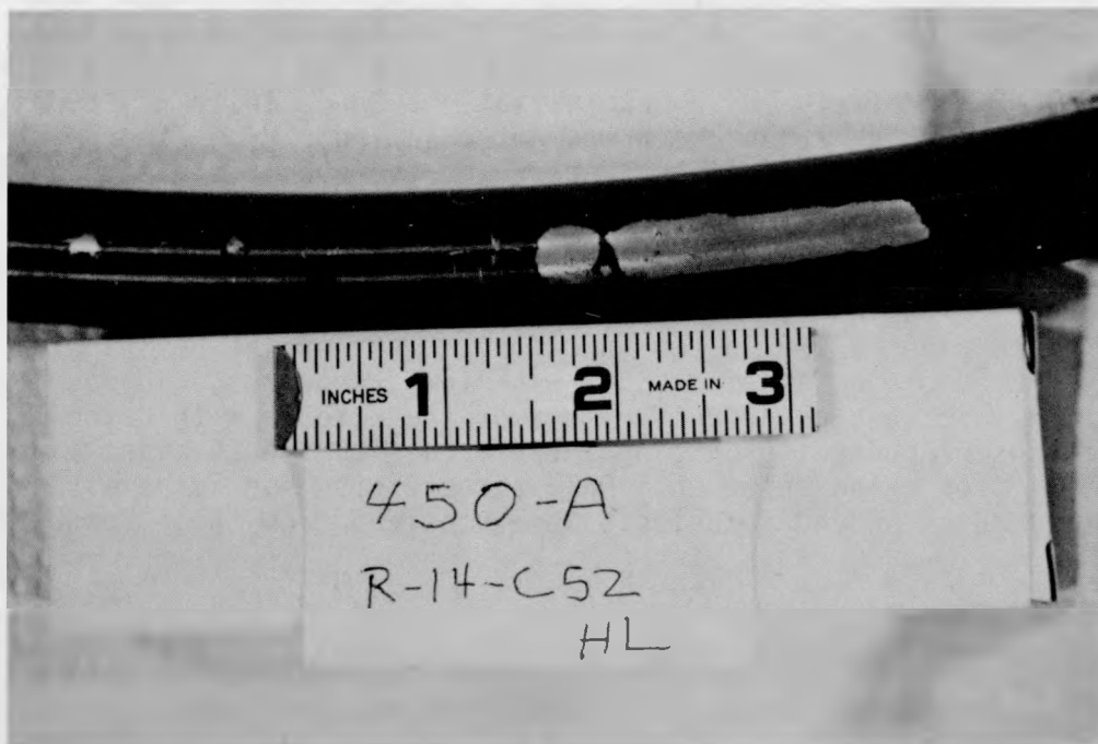
FIGURE 3.29. U-Bend Specimen 450A (R14 C52 HL) Showing Discontinuities in the Copper-Rich OD Surface Deposit
