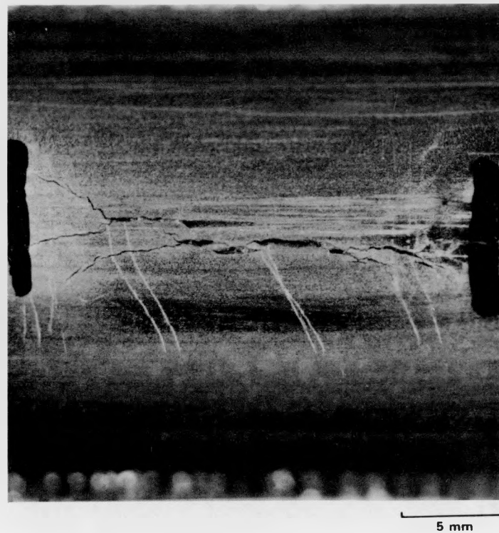
FIGURE 3.31. First TSP Specimen 1041 (R4 C51 HL) Showing ID Cracking (26.9% strain)
