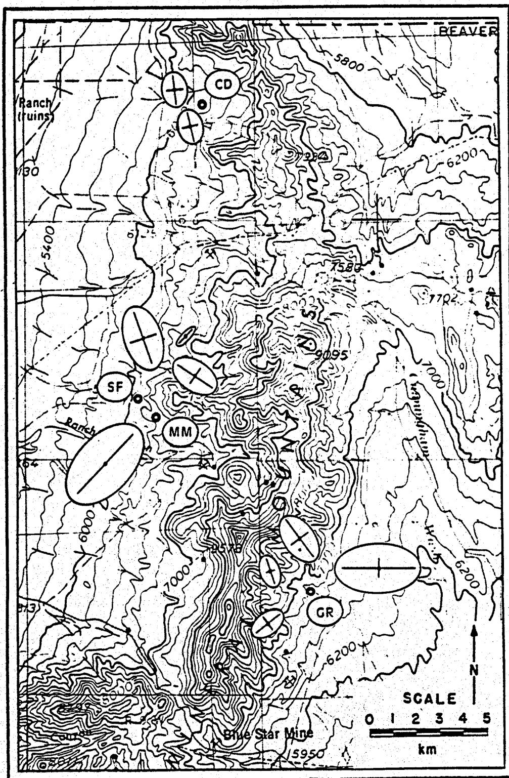
Figure 5: Orientations and magnitudes of principal strains measured in surficial strain-relief tests. For strain-relief axes 1 cm is equal to 250 microstrains.
