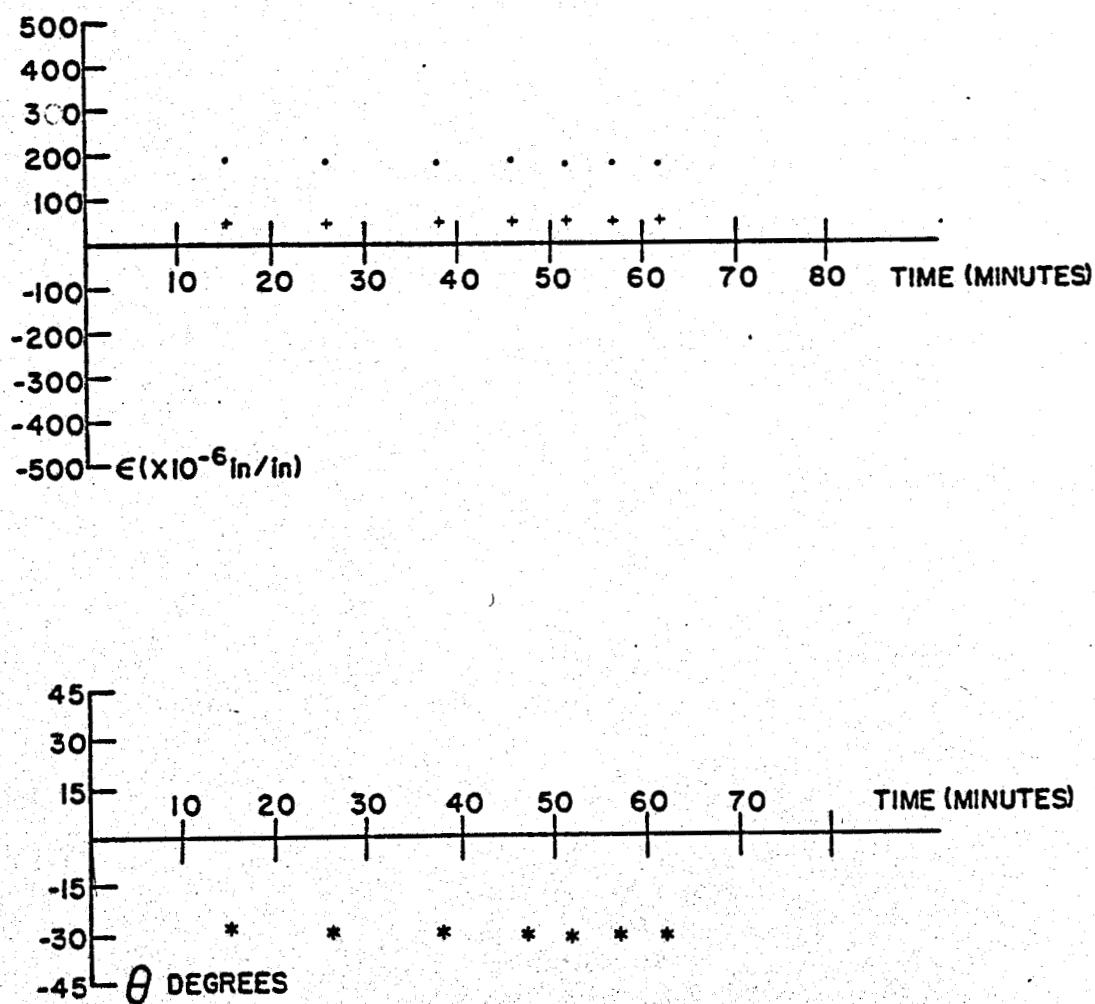
Figure 6: Variations in maximum strain (•), minimum strain (+), and angle between a principle strain and element 3 of the rosette (\*) for test core GR2.
