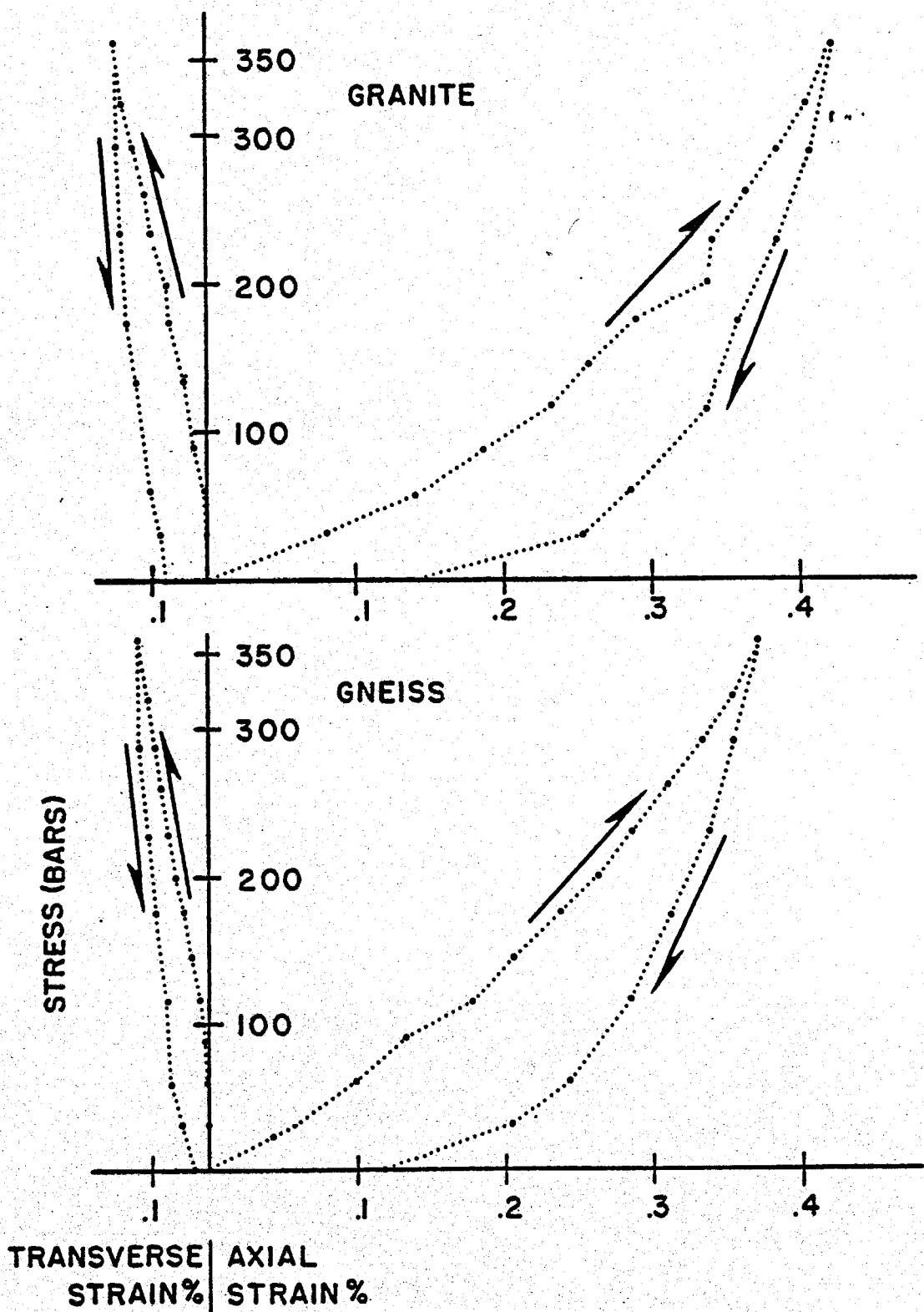
Figure 7: Typical stress-strain curves for uniaxial compression of gneiss and granite cores from the Mineral Mountains.
