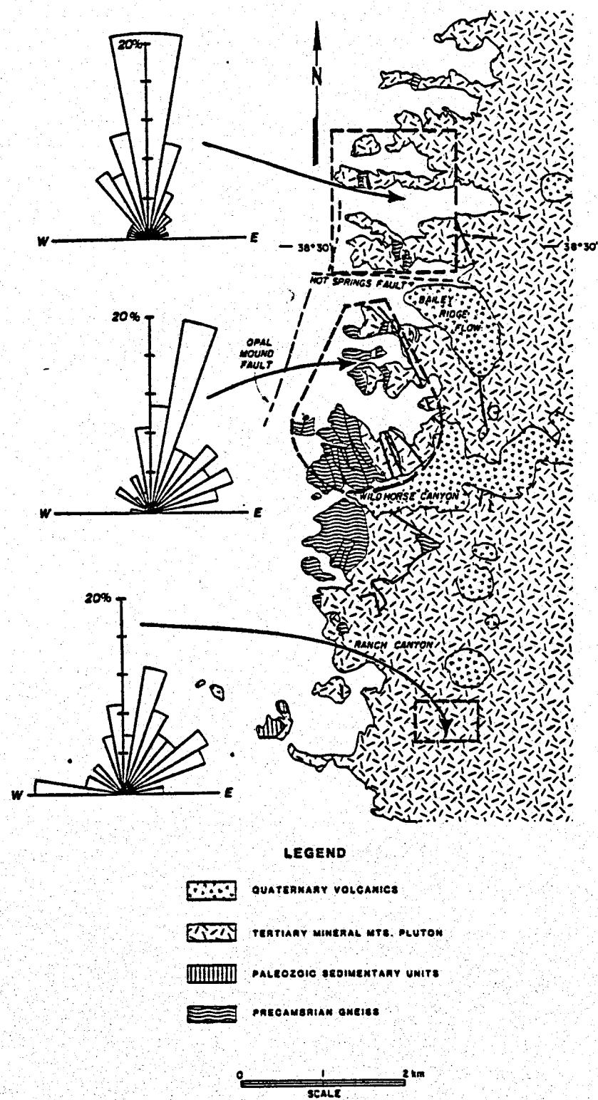
Figure 3: Rose diagrams of strikes of 50 steeply dipping dikes compiled for three regions in the central Mineral Mountains.
