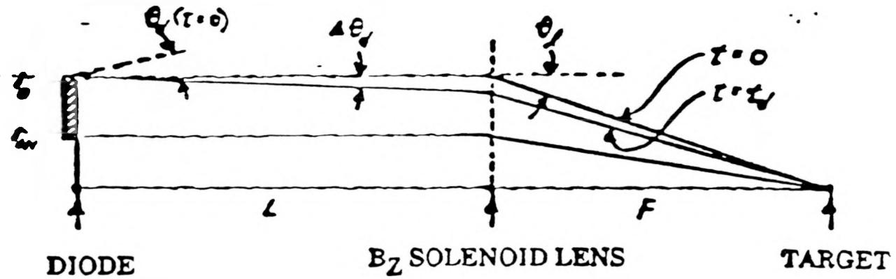
Fig. 8. Achromatic magnetic lens system.
