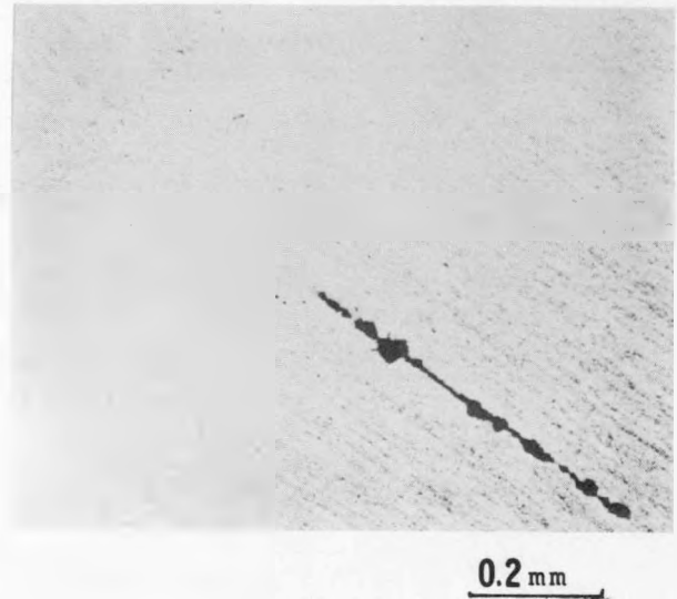
Fig. 7.11.5 Interdendritic shrinkage porosity in 5/8" thick, 200°C preheat Y-groove test weld
