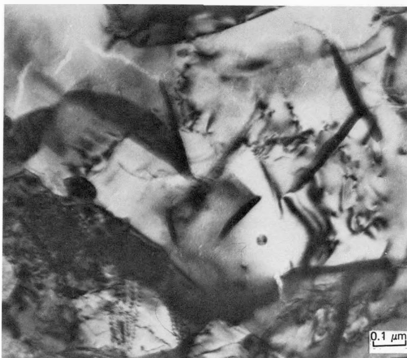
Fig. 7.5.5. Elongated precipitates found in 9 Cr-1 MoVNb after HFIR irradiation at 500°C.
