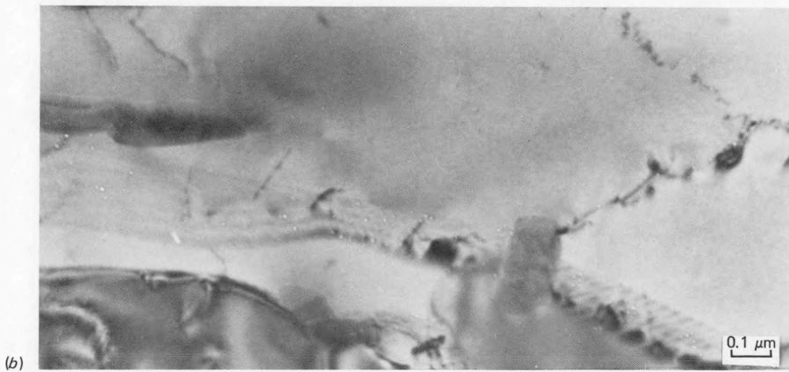
Fig. 7.5.3. Microstructures following HFIR irradiation at 600°C to 4.9 \times 10^{26} neutrons/m 2 in (a) 9 Cr-1 MoVNb and (b) 12 Cr-1 MoVW. Arrows indicate helium bubbles.
