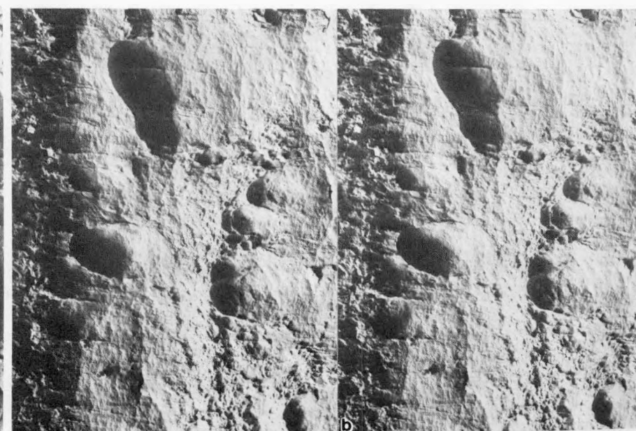
Fig. 7.6.9. Stereo pair fractographs of charpy specimen FA27, 9Cr-1Mo base metal, irradiated to 5 dpa at 55°C in HFIR and tested at 85°C (a) at low and (b) intermediate magnification.
