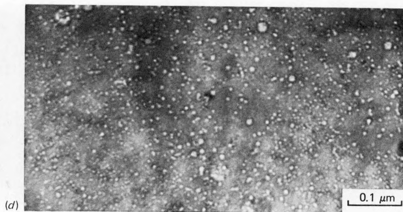
Fig. 3.1.4. Cavity microstructures of PCA-A3 irradiated in HFIR to ~44 dpa at (a) 300°C, (b) 400°C, (c) 500°C, and (d) 600°C. Note the void formation at 500°C.
