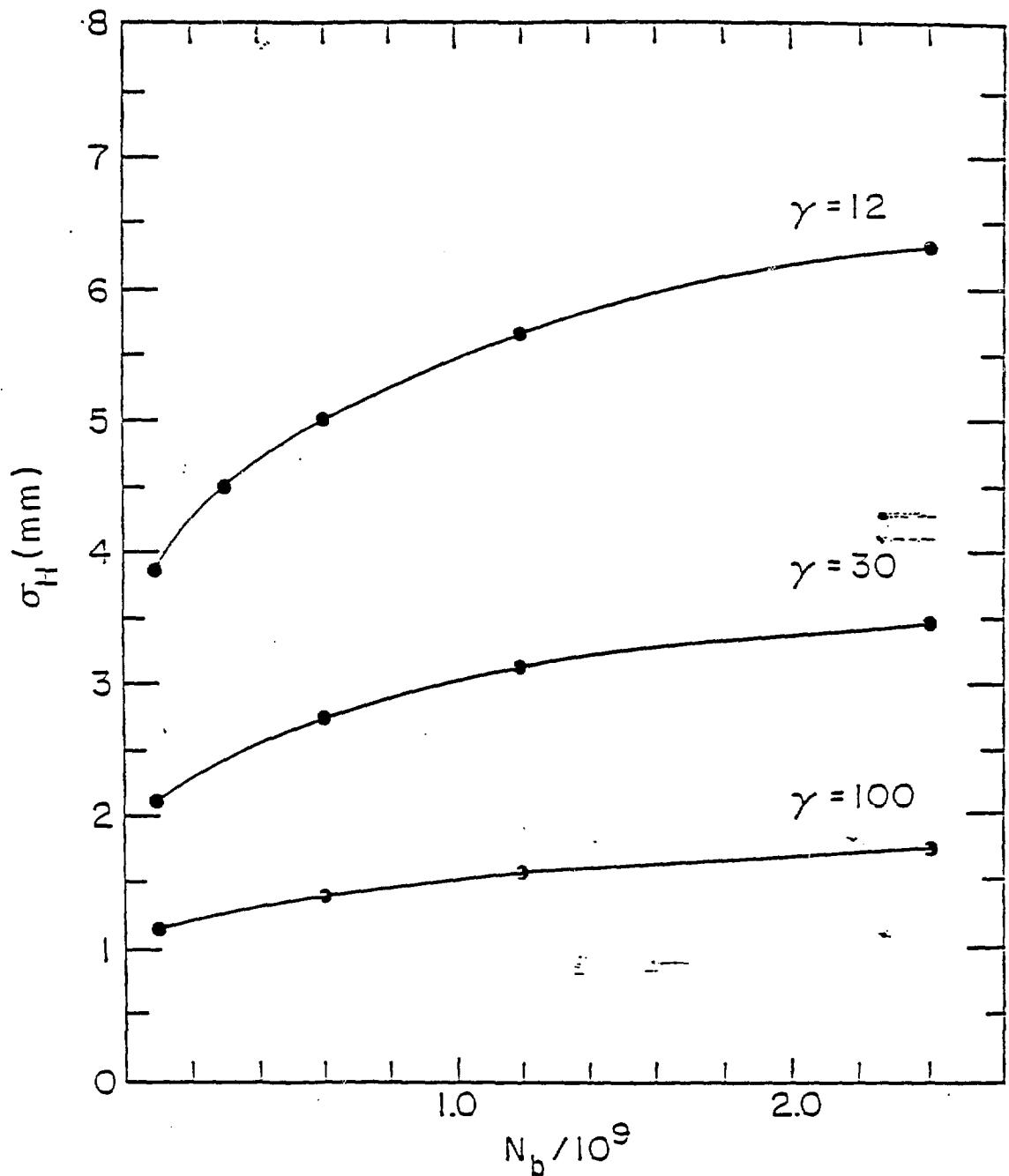
Results for a beam of gold ions showing the effects of coupling on the beam growth due to intrabeam scattering.
