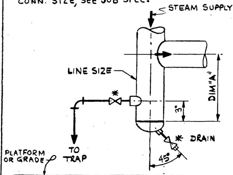
**DETAIL-2** AT C.V. MANIFOLD OR STEAM INLET TO TURBINE
