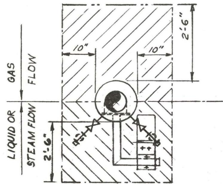
LEAVE SHADED AREAS CLEAR FOR MOUNTING OF SEAL POTS, INSTRUMENT ETC.
