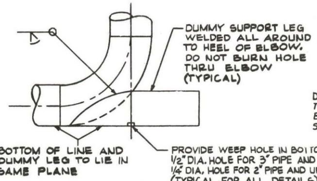
DUMMY LEG FOR ALLOY LINES THIS APPLICATION SHOULD BE USED ONLY WHEN SPECIFIED ON PIPING DWG.
