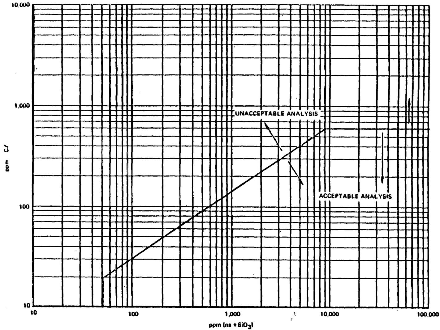
Figure 1 - Acceptability of insulation material on the basis of the plot points of the Cl and the (Na + SiO<sub>3</sub>) analyses.
