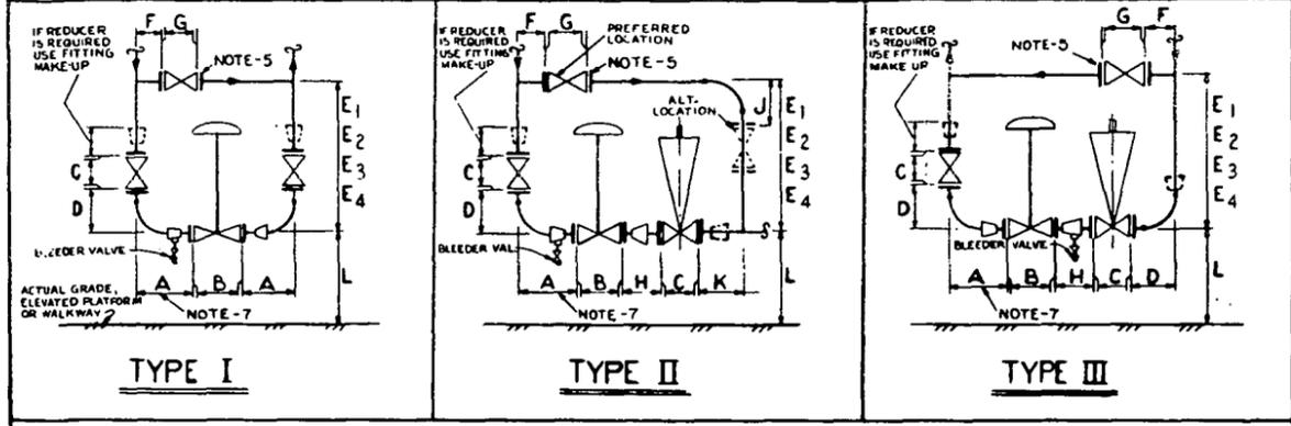
SCREWED AND/OR SOCKET WELD MANIFOLDS
