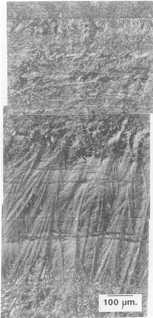
Figure 25. Optical micrograph (differential interference contrast) of the solder film on a gold-nickel-plated Kovar sample on which no flux was employed.
