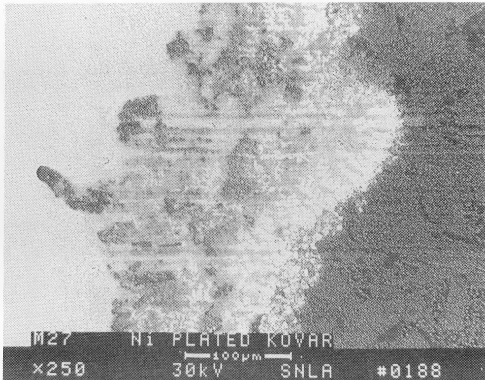
Figure 21. SEM micrograph (backscattered electron) of the solder-film edge on a nickel-plated Kovar sample fluxed with B1452. The solder-film is to the left; the plated surface to the right.
