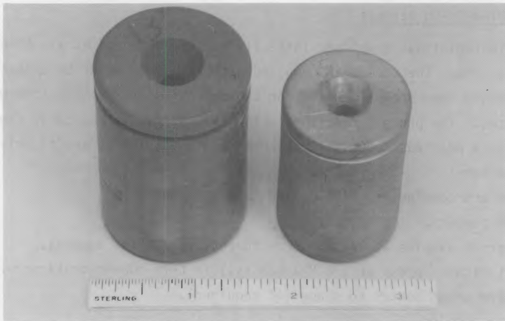
FIGURE 1. NiO-NiFe 2 O 4 -Cu (17 wt% Cu) Anode Before (on left) and After (on right) Sintering
