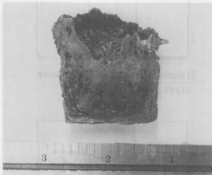
FIGURE 8. Anode That Failed Due to Severe Corrosion (from Experiment 25)
