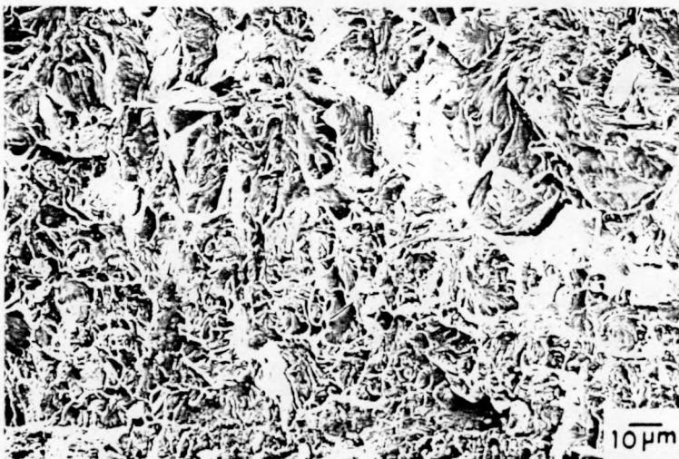
Figure 30. SEM Photographs for Fracture Surface of 9 Cr-2WV Steel after Final Bending: (a) Total Section (b) Center Coarser Grain Structure Region (c) Finer Grain Structure Region.
