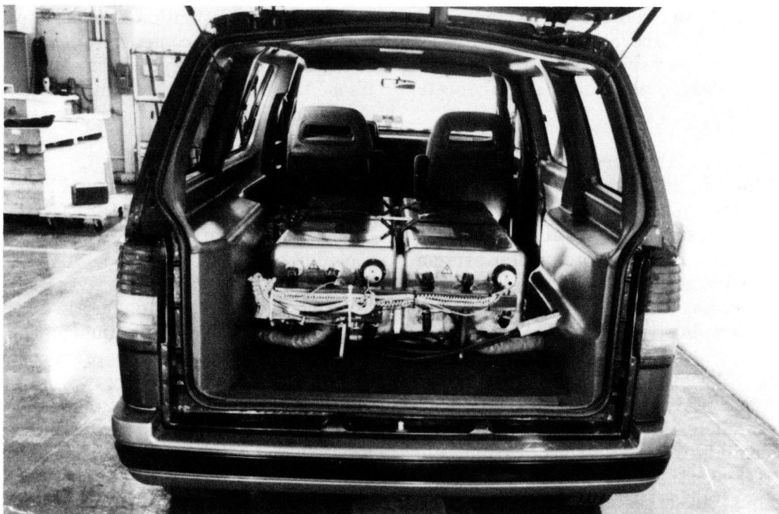
Figure 8: ETX-II With two B-11 sodium sulfur batteries
