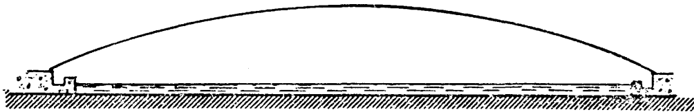
Fig. 2. Inflated plastic cover design
