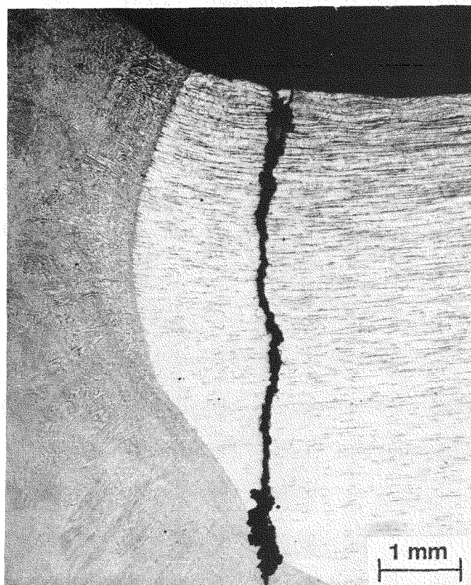
Figure 14. Portion of Metallographic Section OB (Fig. 12) Showing Crack Extending from ID Surface into Test Weld.
