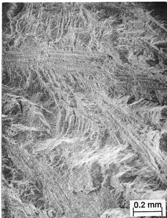
Figure 15. SEM Fractograph on Specimen from Section OA (Fig. 12) Showing Presence of Fatigue Striations (Center of Photograph) on Fracture Surface.
