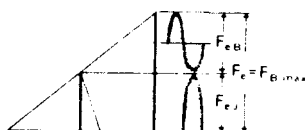
Figure 25. Joint diagram shows how insufficient preload F_i causes excessive additional bolt load, F_{eB} .
