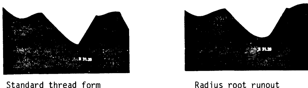
Figure 16. Comparison of a standard thread form and the radius root runout.
