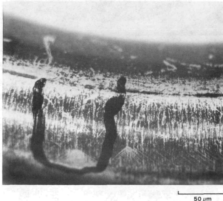
FIGURE 3.9. Axial and Circumferential Cracking on the OD Surface at the Apex of U-Bend Specimen 1049B (R2 C27)
