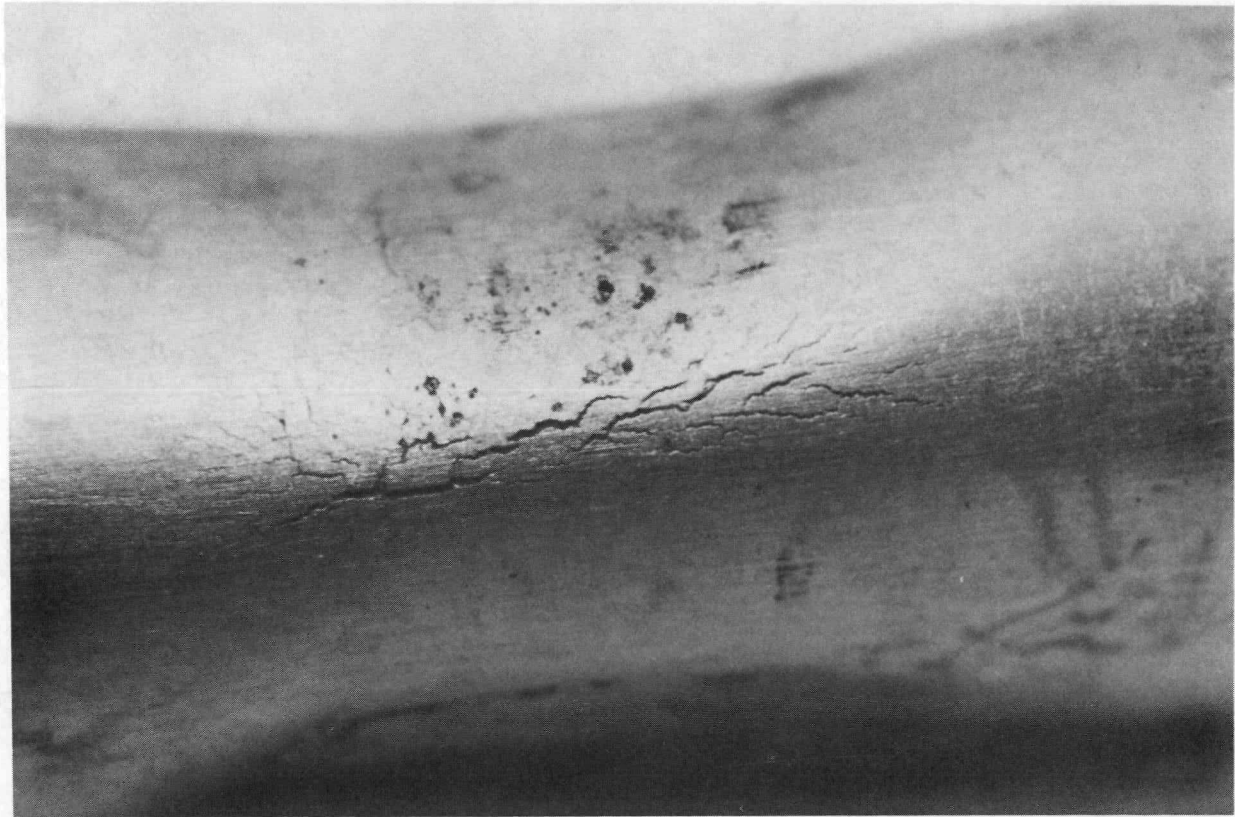
FIGURE 3.24. Photograph Showing Axial Cracking of Seventh TSP Specimen 451 (R45 C50 HL7) (79.8% strain)
