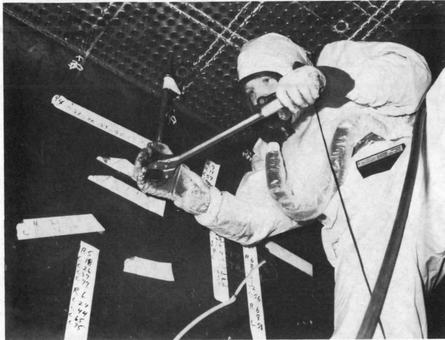
FIGURE 2.8. Cutting TTS Specimen Above the Sludge Pile
