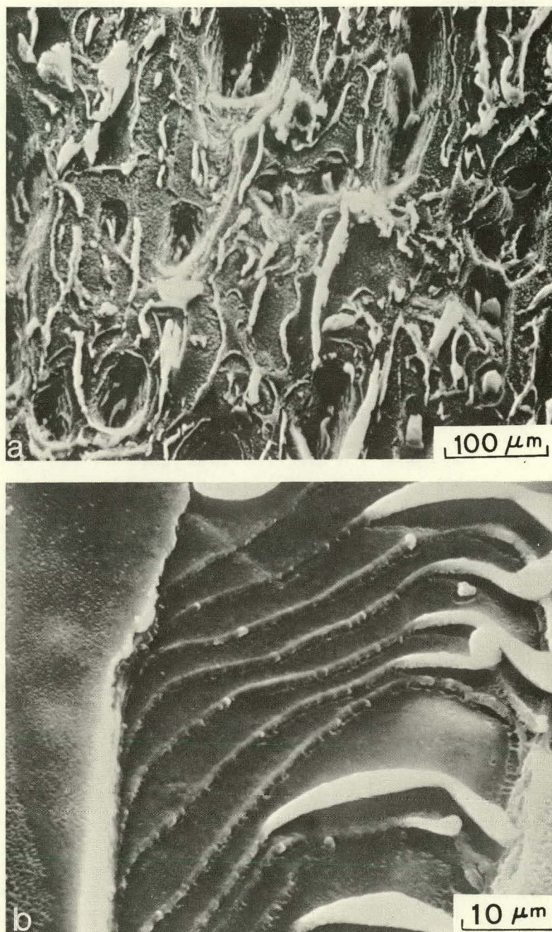
Figure I-3. (a) Scanning electron micrographs of annealed polycrystalline aluminum irradiated at 250°C with 100-keV ^4\text{He}^+ to a total dose of 1.2 \times 10^{20} ions/cm 2 . Figure I-3(b) is an enlarged view of an area in Figure I-3(a) showing multiple exfoliation of blister skins.
