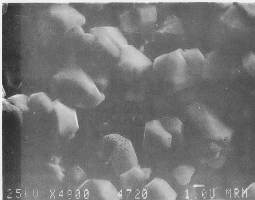
Figure 30. High magnification SEM photograph of 3-layer CdS film fired at 653°C for 100 minutes, originally containing 40 volume percent CdCl 2 .
