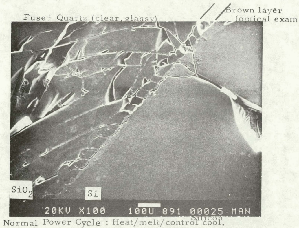
Figure 14. SEM Examination of Silica/Silicon Interface
