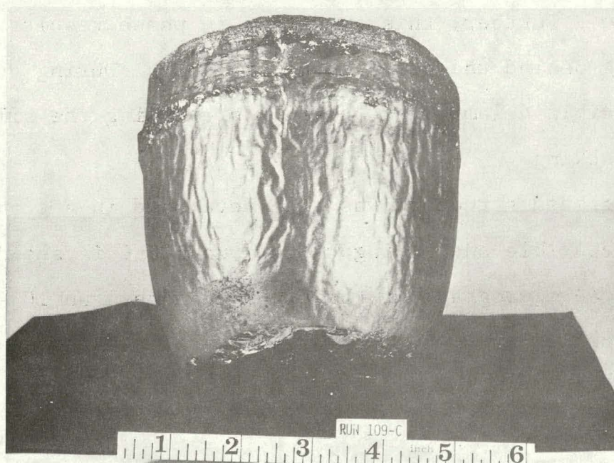
Figure 26. Crack-free 3.3 Kg Silicon Boule Cast in Run 109-C
