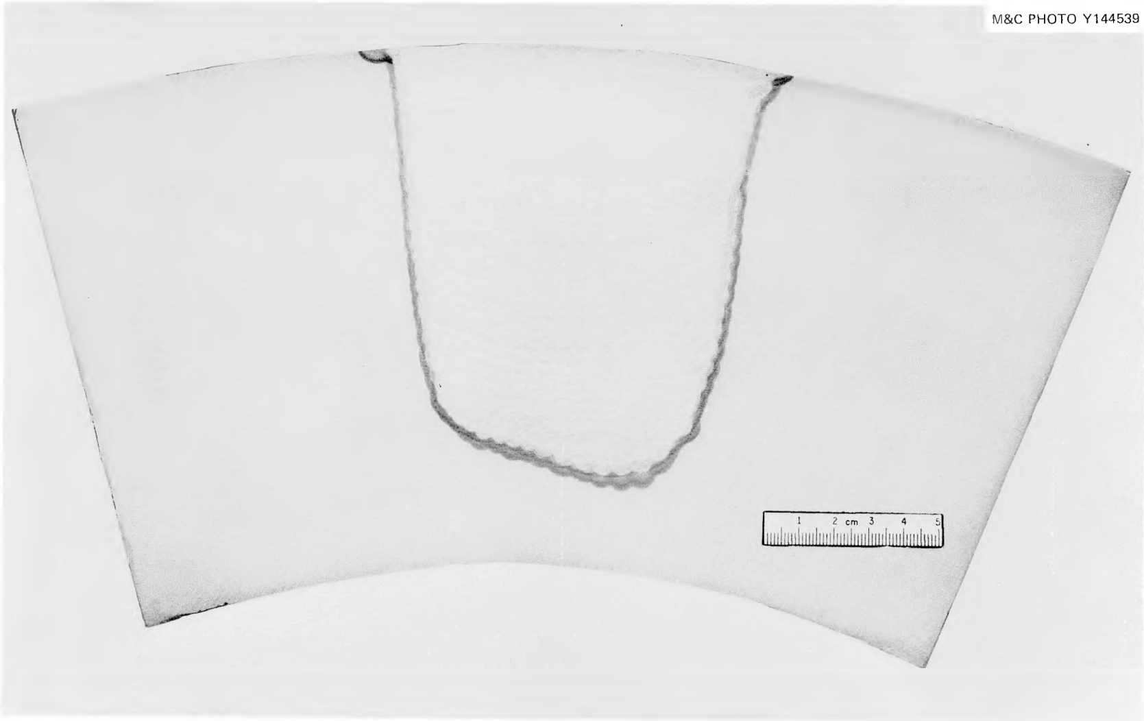
Fig. 2.9. Cross section of the prototypical half-bead weld repair for vessel V-7B. The sides of the cavity in this piece are more irregular than in the vessel because the V-7B cavity was not machined.
