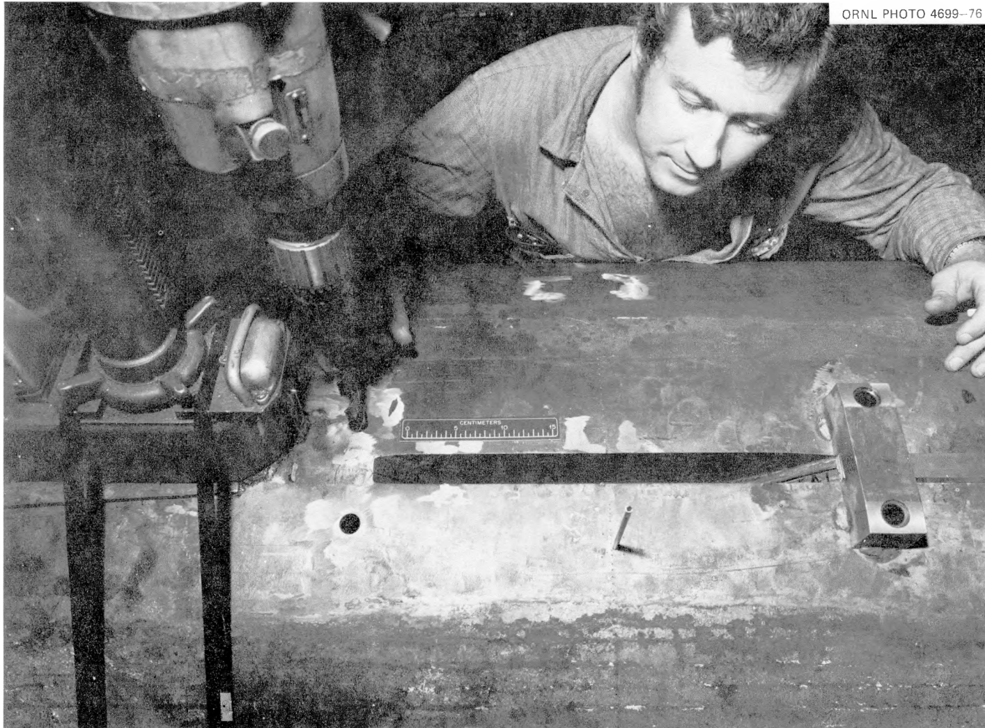
Fig. 2.2. Removal of the flaw region from vessel V-7A after the test. Drilled holes mark the corners of the block flame-cut from the vessel.
