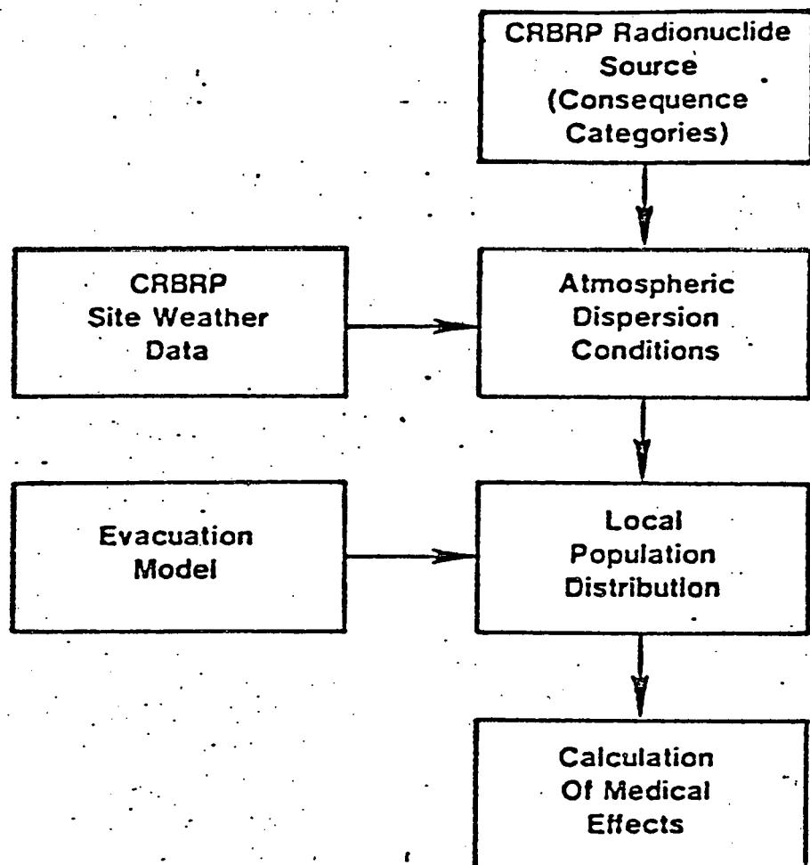
Figure 3. Schematic View of Consequence Calculational Model
