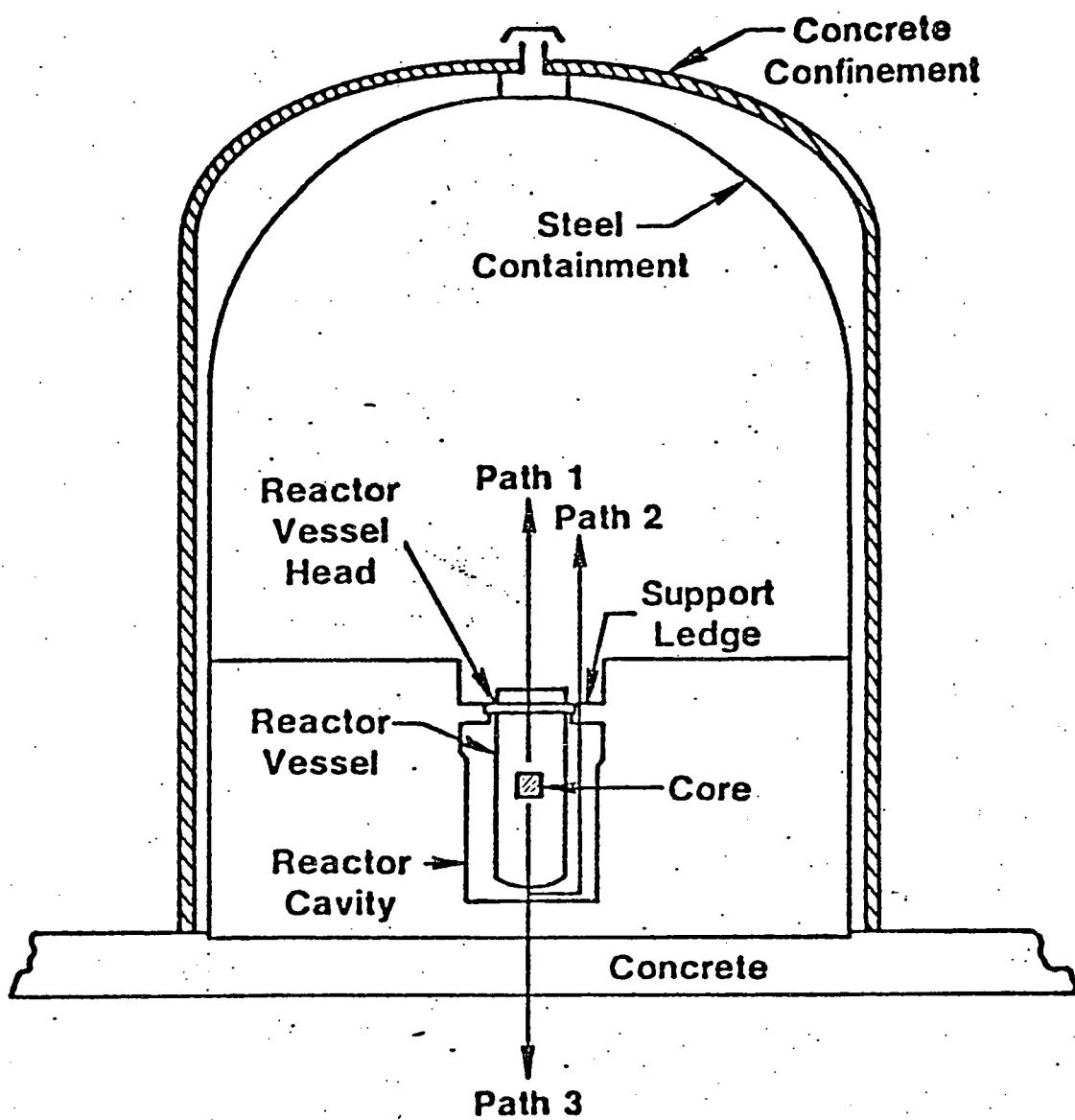
Figure 1. Schematic Diagram of Post-CDA Radionuclide Flow Paths
