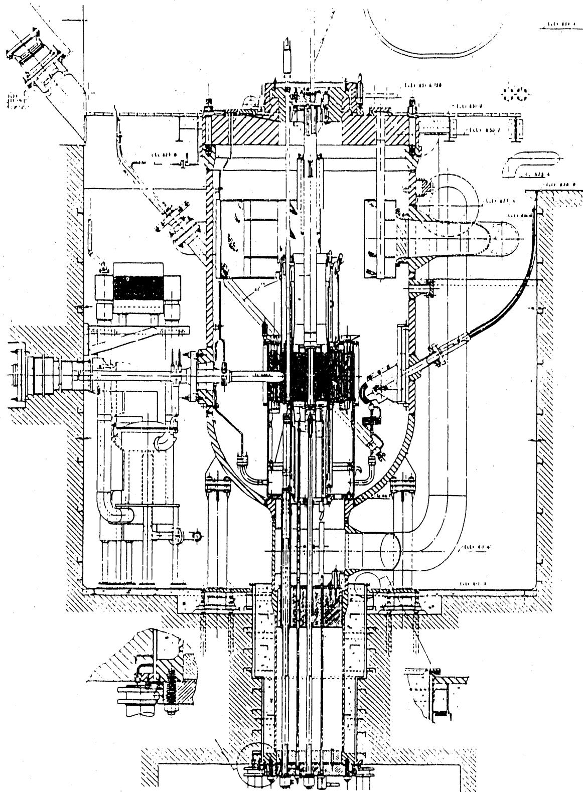
Fig. 1. Vertical Section of HFIR Reactor Vessel and Core
