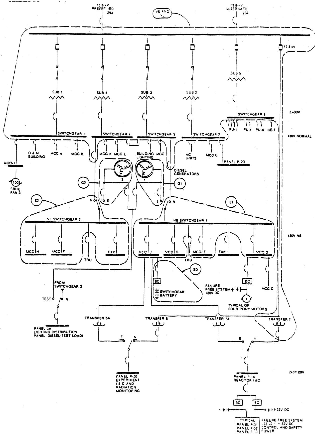
Fig. 3. HIFIR Electrical System Schematic
