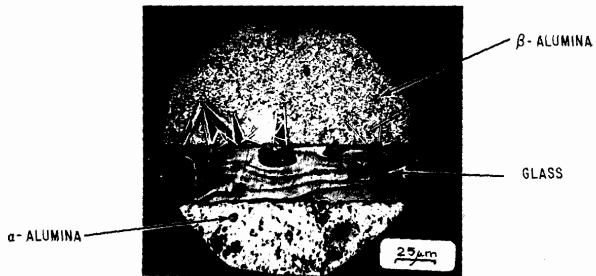
Figure L.12. Cross-section of Beta-alumina/Glass/Alpha-alumina Seal
