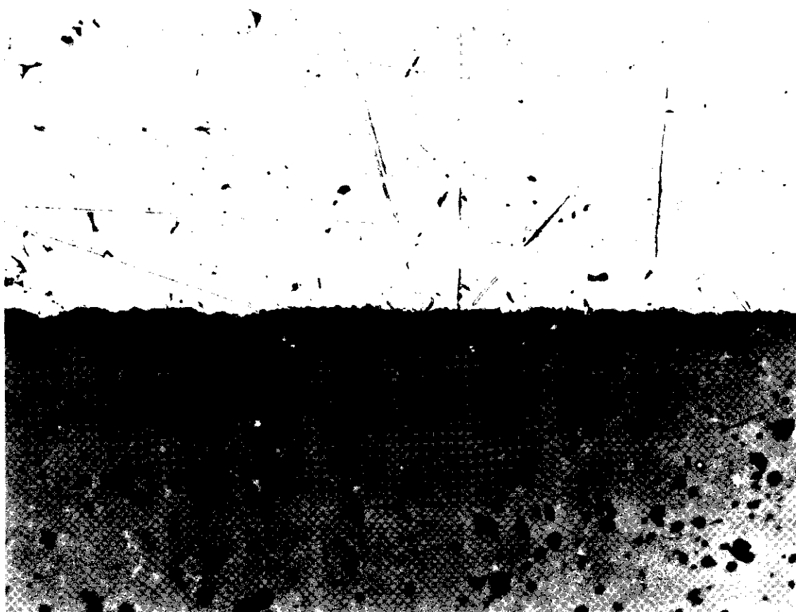
Figure E.2. Aluminum/Alpha-alumina Interface of a TCB Seal (500X)
