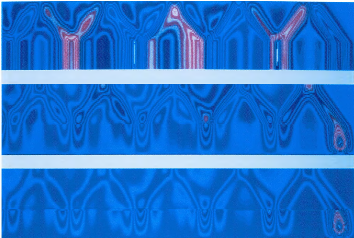
Figure 7: Longitudinal Electric, Azimuthal Magnetic, and Radial Electric Fields (from top-to-bottom) of the Wakefield Accelerator
