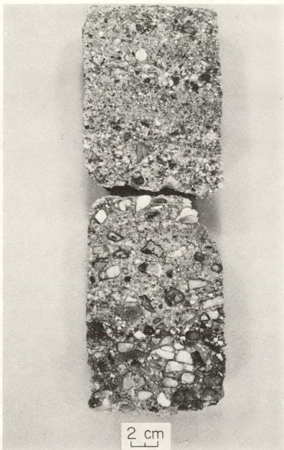
Figure 18a. Upward-fining sequence in granite wash from Standard and Robinson #2 Tippen well, Cottle County. Depth is 2,080.6 m (6,826 ft).
