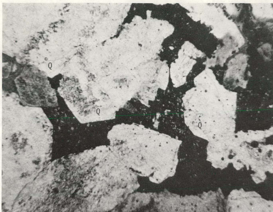
Figure 35. Euhedral quartz overgrowths (Q) in Standard and Robinson #2 Tippen well, Cottle County; depth 2,074.5 m (6,806 ft).
