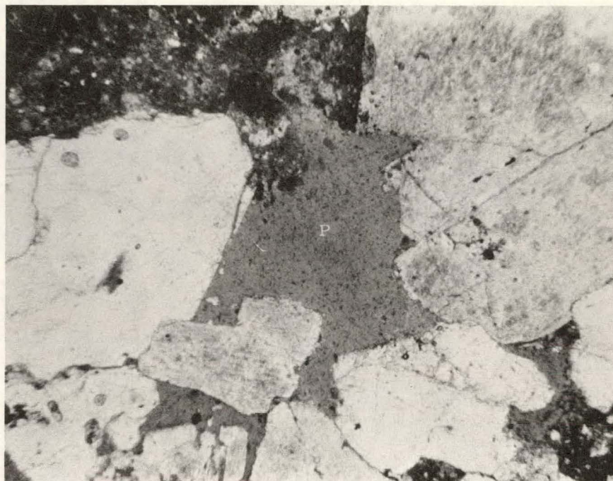
Figure 37. Secondary porosity (P) in Standard and Robinson #2 Tippen well, Cottle County; depth is 2,074.5 m (6,806 ft).
