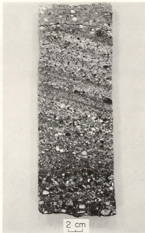
Figure 18b. Crossbedding in granite wash, Standard Oil #1 Barron well, Cottle County. Depth is 1,995.2 m (6,546 ft).
