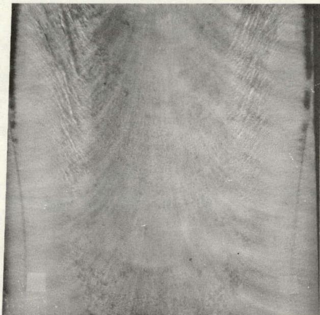
FIGURE 18. Low-Energy Radiograph of a Section Through the Center of an Ingot
