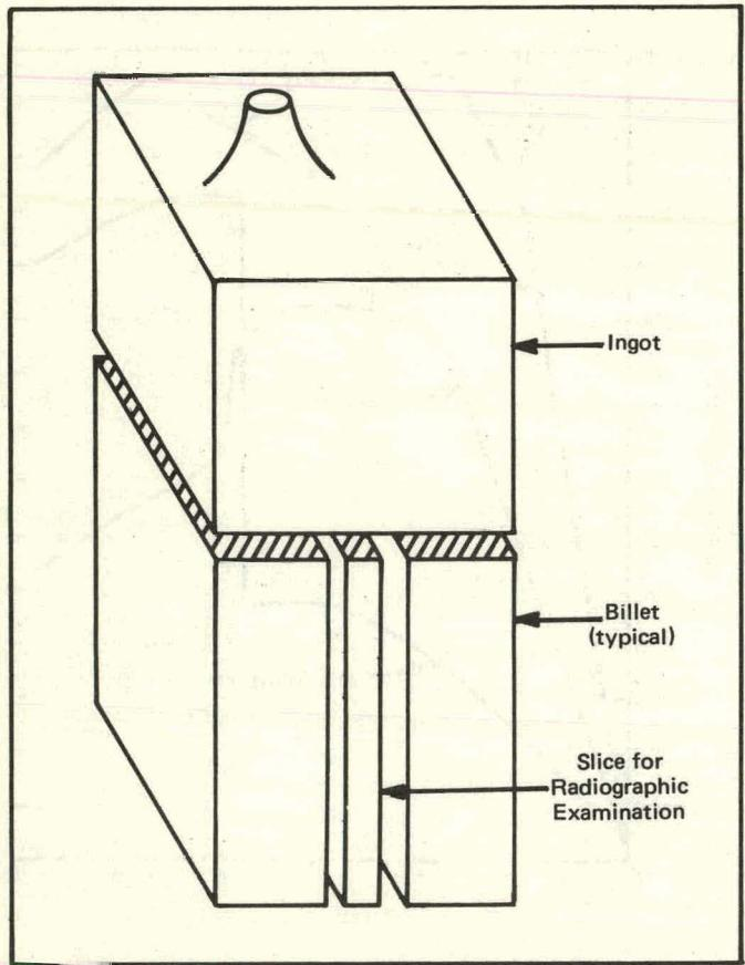
FIGURE 16. Ingot Area From Which the Two Billets for Sheet Rolling and the Slice for Radiographic Inspection Were Sectioned. The Top Portion of the Ingot Was Returned to Feed Stock.
