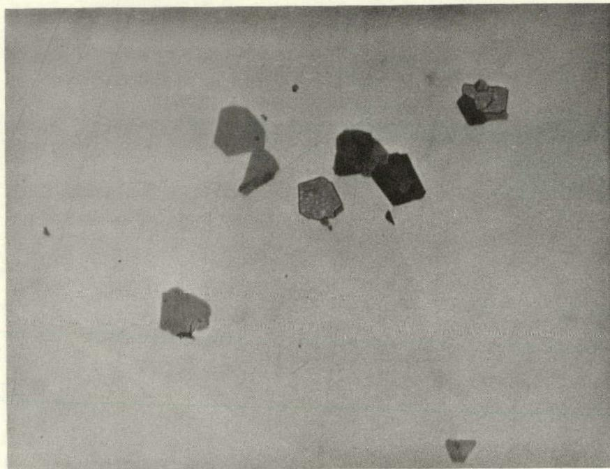
FIGURE 24. Typical Beryllium Carbide Inclusion Found in Ingots (600X)
