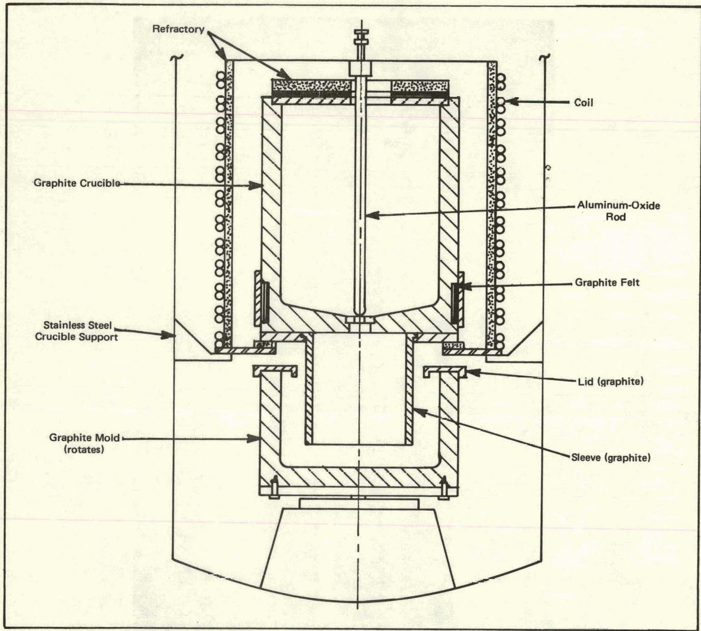
FIGURE 13. Centrifugal Casting Assembly.
