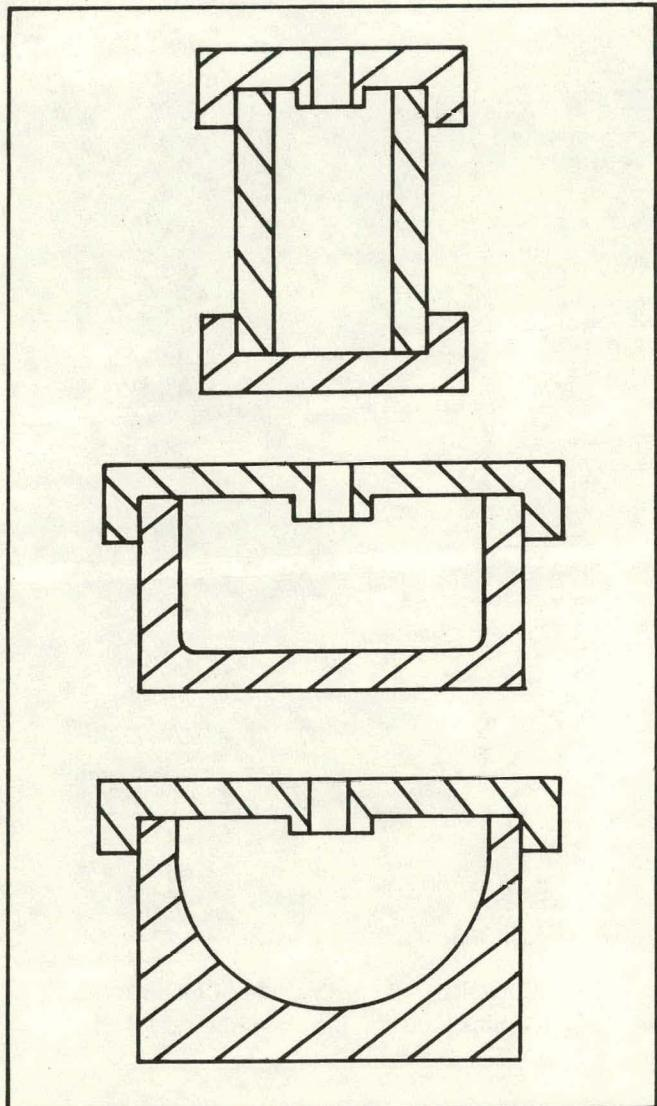
FIGURE 14. Centrifugal Casting Molds
