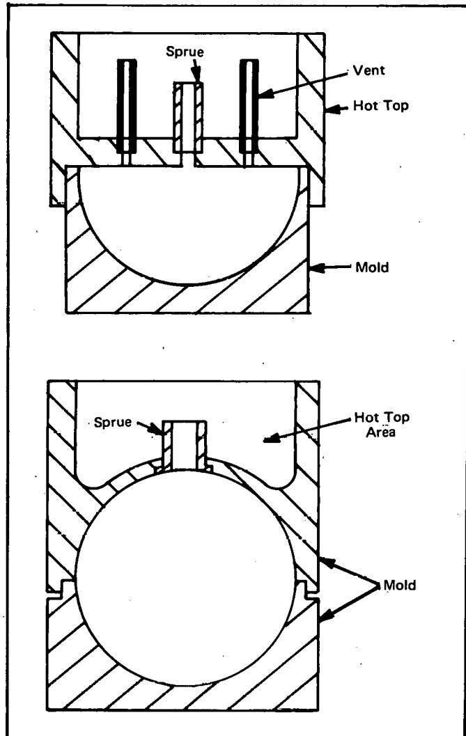
FIGURE 6. Molds and Hot Tops Used for Casting 11.5- to 44.6-cm Spheres and Hemispheres
