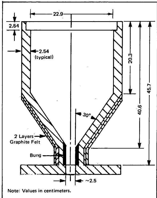
FIGURE 2. Tapered Crucible
