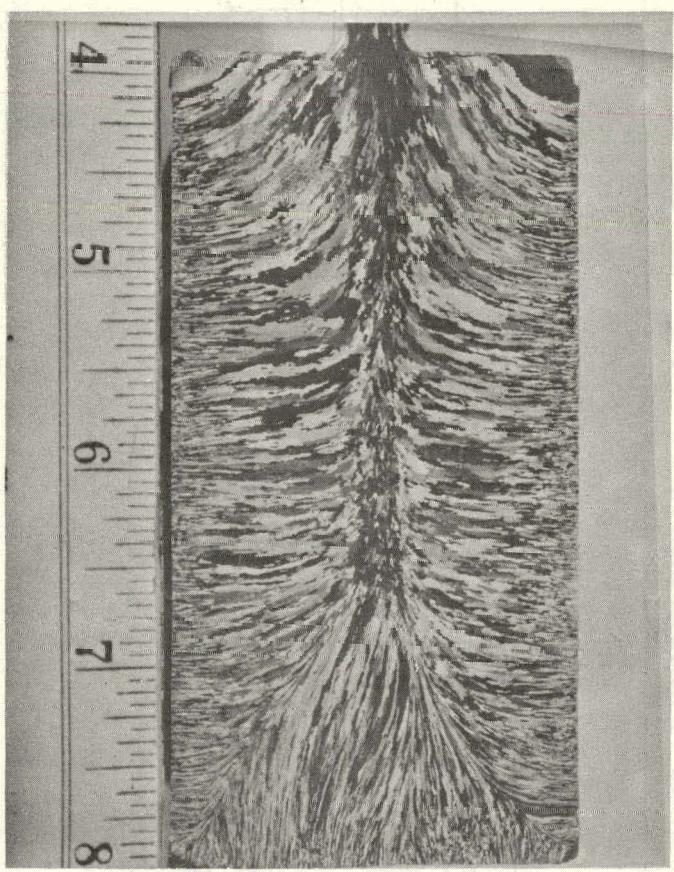
FIGURE 17. Typical Columnar Grains Found in Cast Beryllium Ingots
