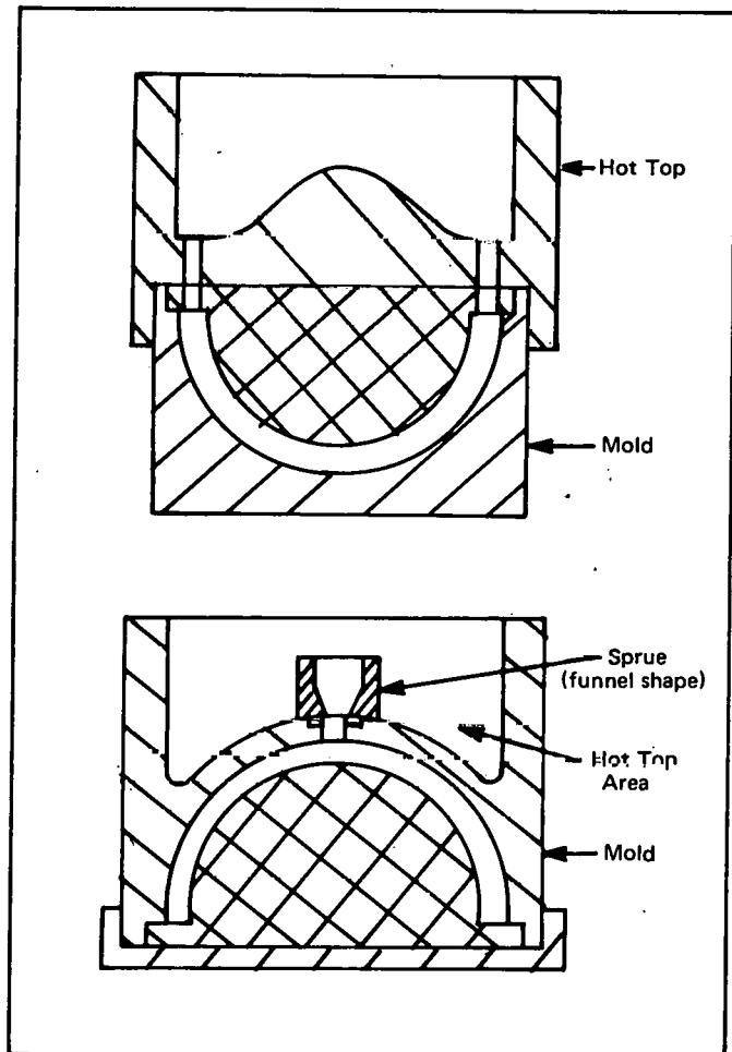
FIGURE 7. Two Types of Hemispherical Molds Used with Limited Success
