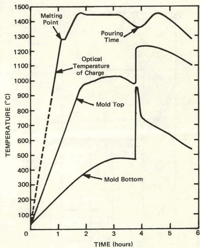
FIGURE 15. Thermal Cycle Used in the Vacuum Induction Casting of Beryllium at Rocky Flats. The Temperature of the Charge is Used to Control Power Input and the Temperature of the Mold Depends Upon the Position of the Mold Within the Induction Coil. (Reference 2)
