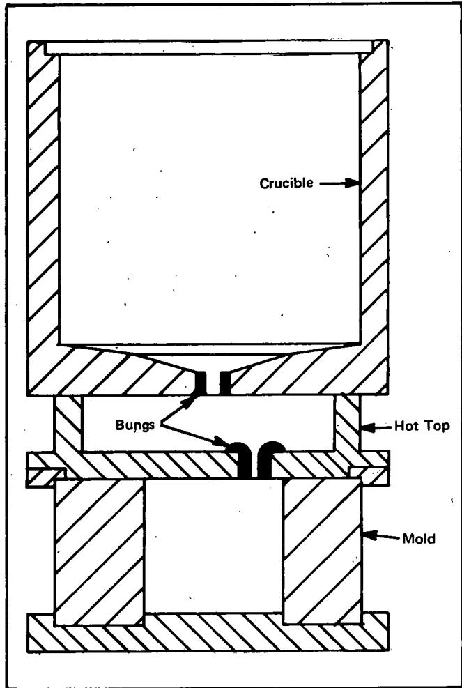
FIGURE 4. Relationship Between the Crucible, Hot Top, and Production Mold
