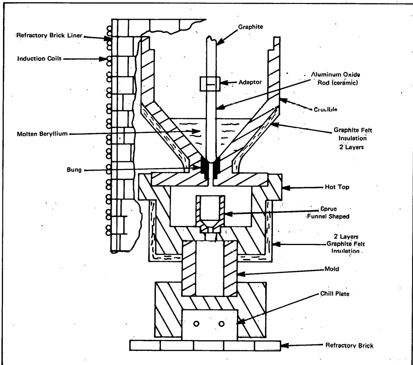
FIGURE 11. Casting Setup Used for Casting Small Research Ingots.
