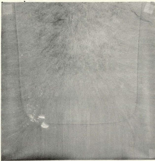
FIGURE 21. High-Density Inclusion in the Left-Hand Corner of the Ingot—Along the Chill Line
