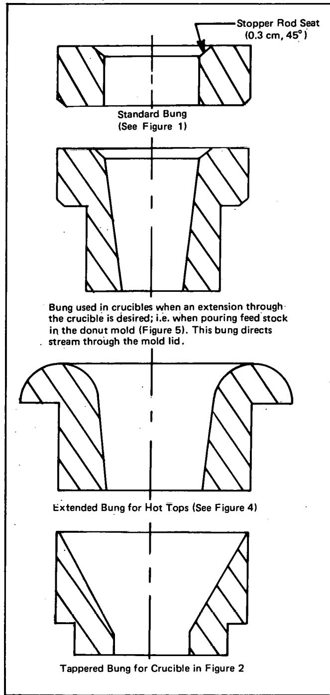
FIGURE 8. Common Bungs Used in Casting Beryllium
