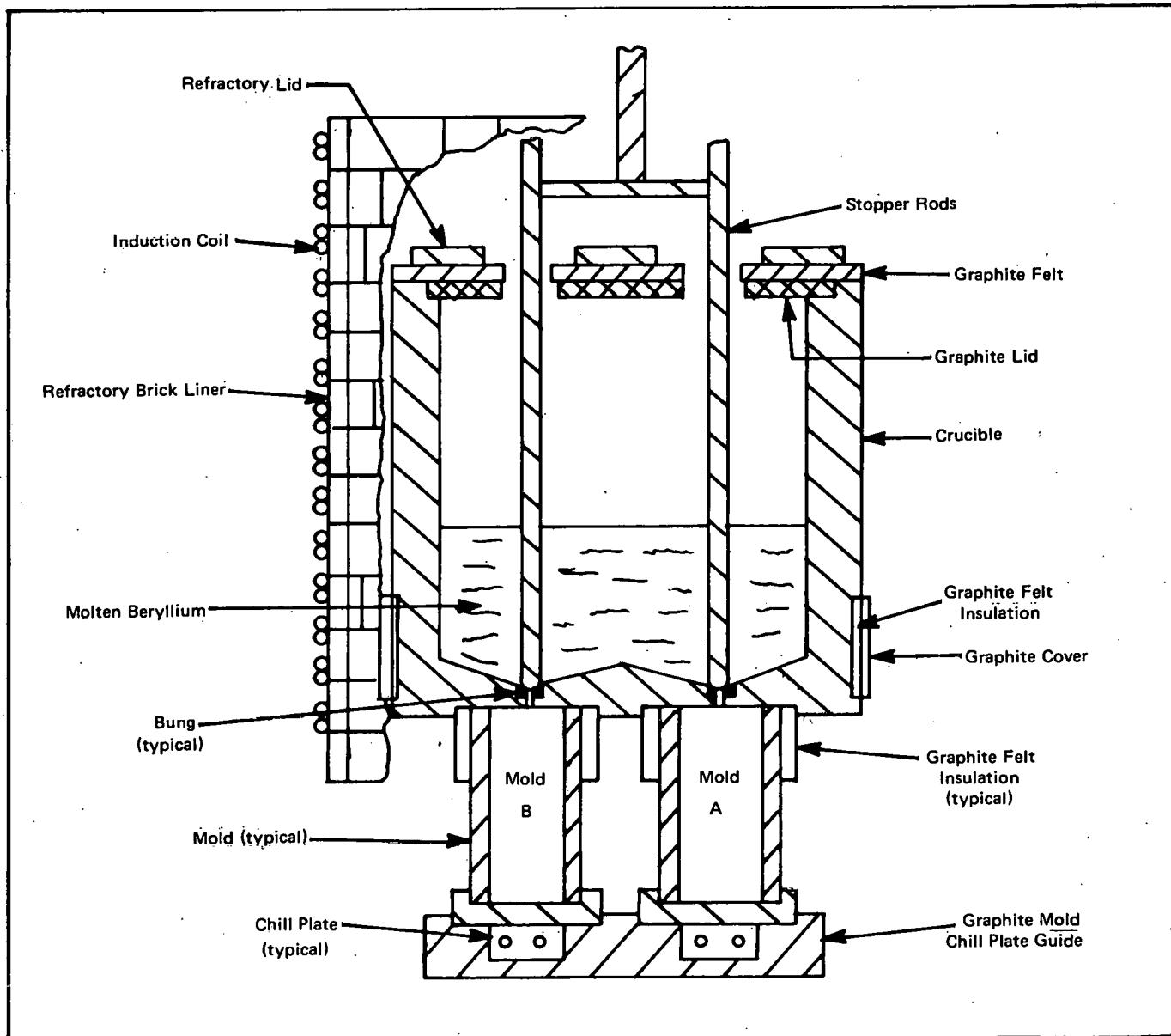
FIGURE 10. General Setup for Tandem Casting. Hot Tops Such as the One Illustrated in Figure 9 May Be Used in This Casting Operation.
