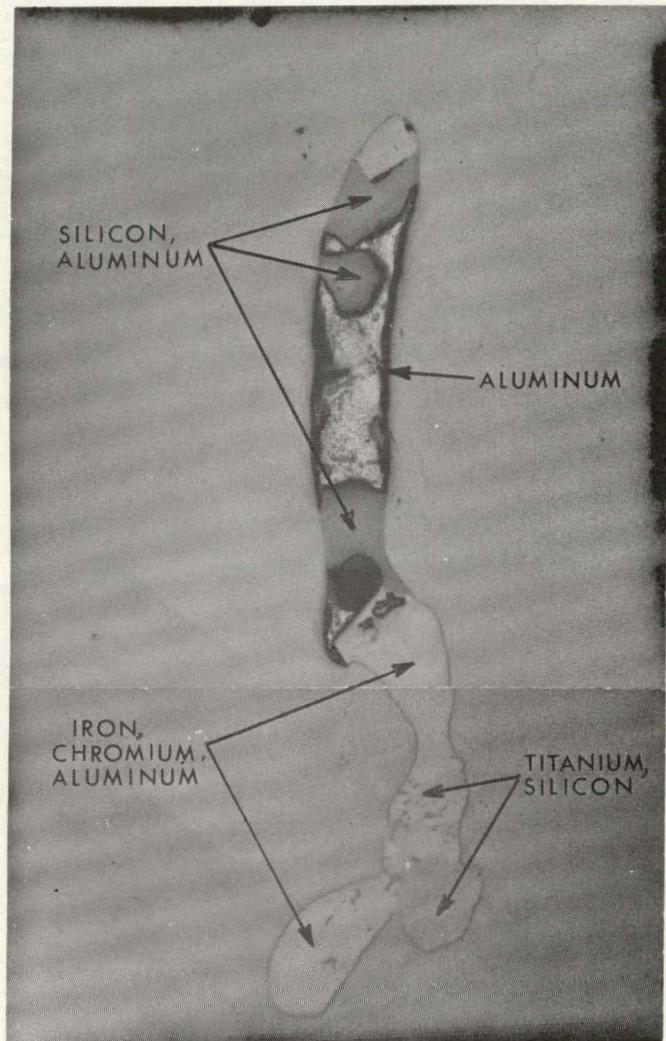
FIGURE 19. High-Density Stringer Found in a Beryllium Ingot. Qualitative results of the major impurity phases are identified. (330X)
