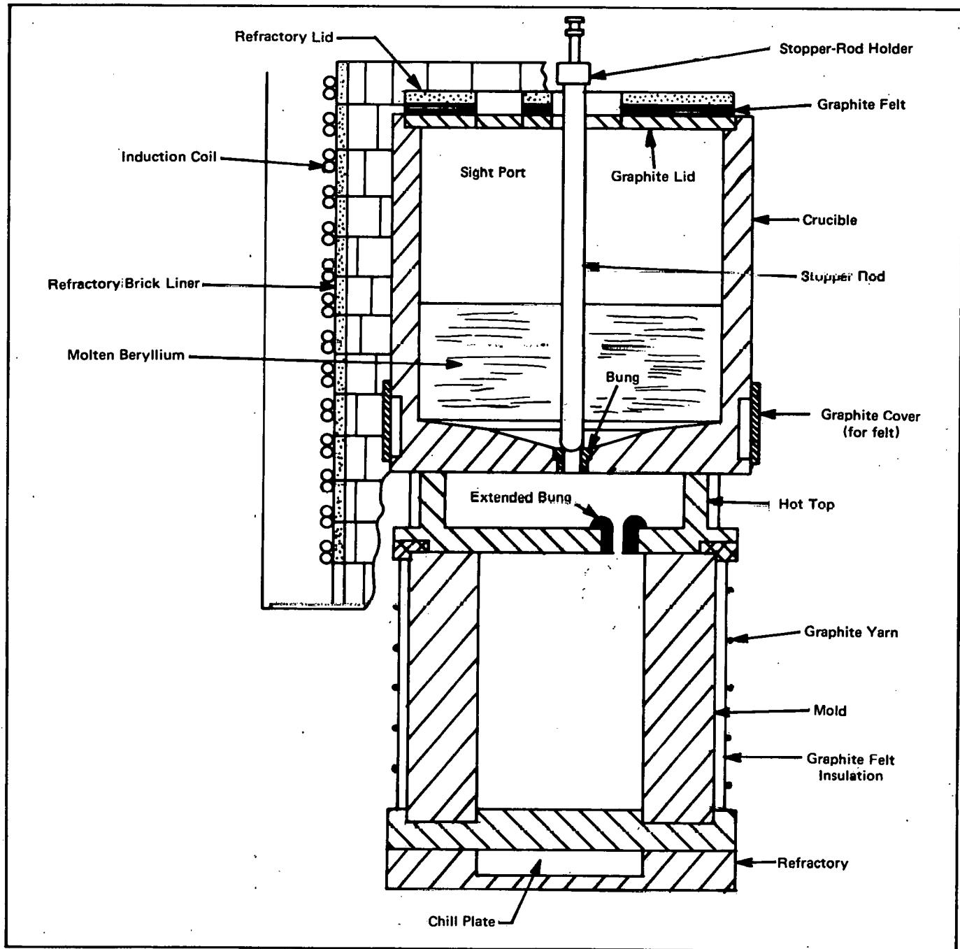
FIGURE 9. Cross - Sectional View of the Mold - Crucible Arrangement Used to Cast Large Beryllium Ingots
