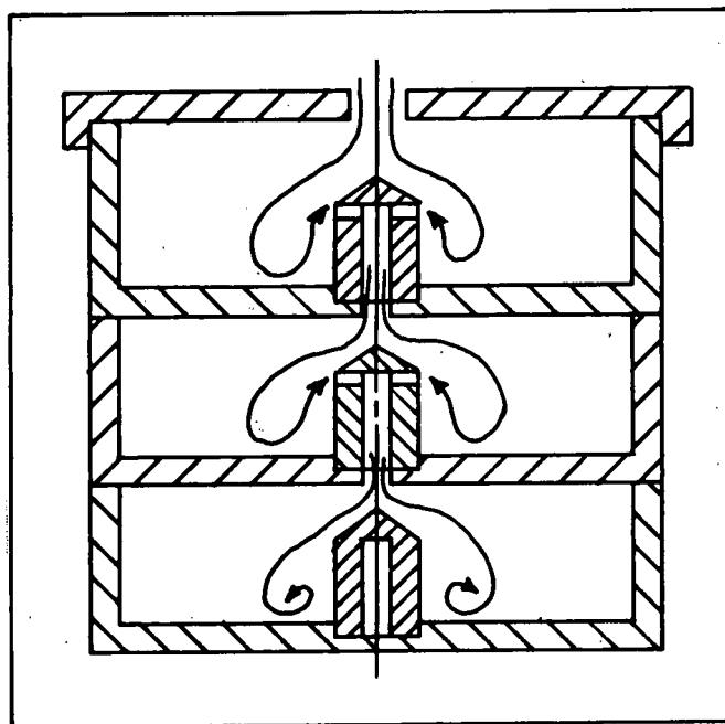
FIGURE 5. Feed Ingot Mold Setup. The Number and Size of the Molds Are Variable. Arrows Indicate Metal Flow.
