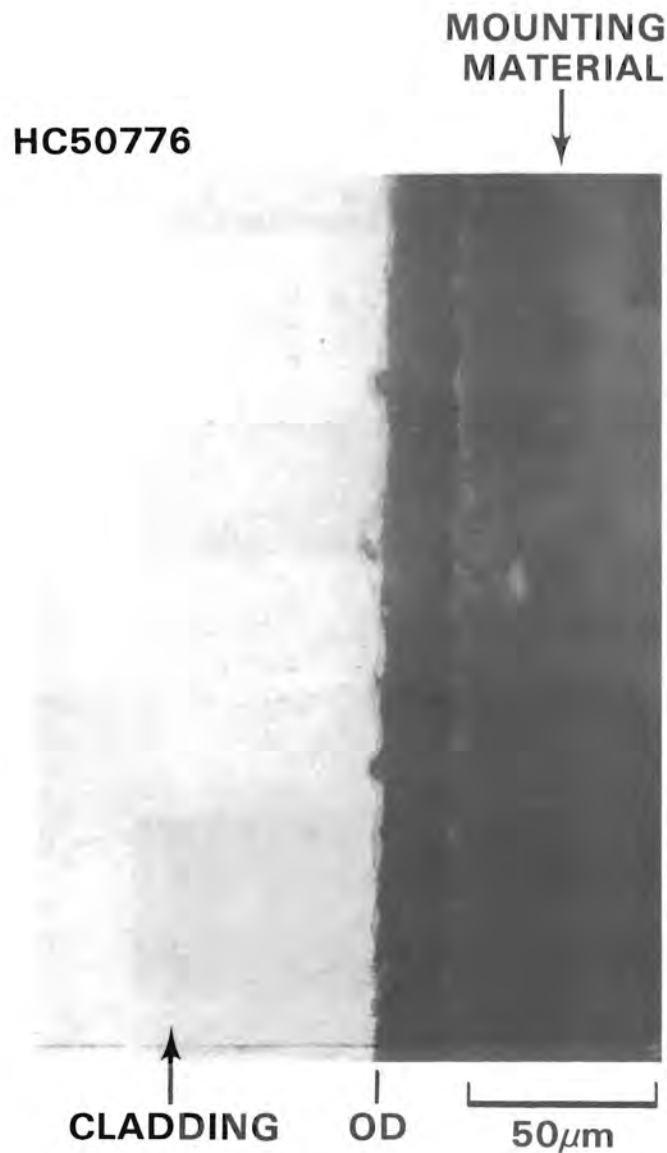
FIGURE 48. Metallography of Surface Layer on Cladding from S004 Fuel Rod AHR
