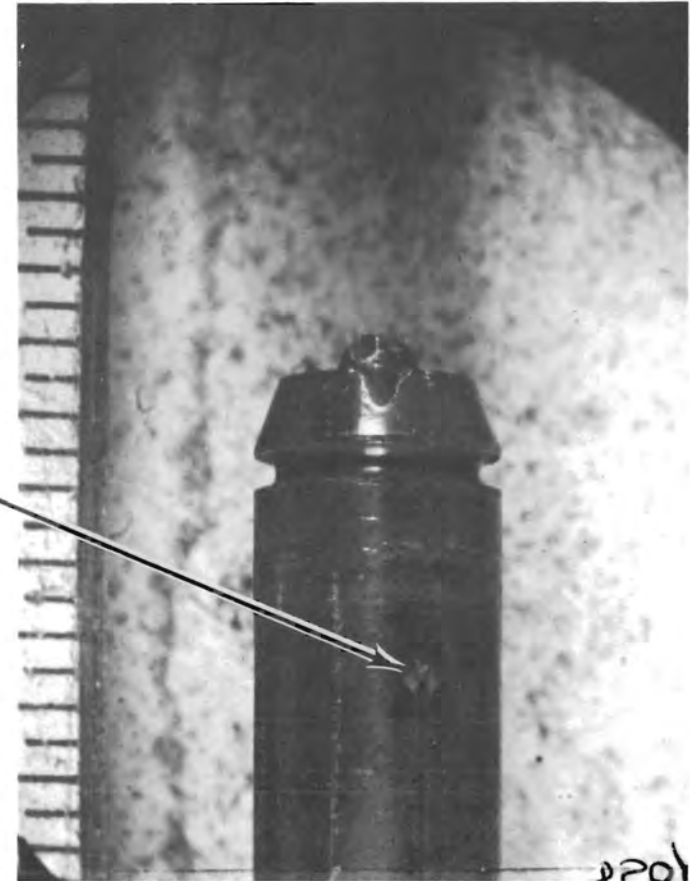
FIGURE 18. Shallow Indentation on Cladding at Grid Spacer Contact Point That was Observed During Visual Examination
