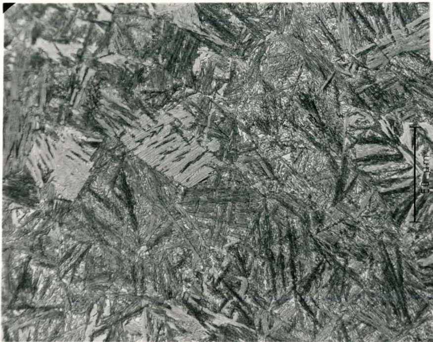
Figure 8. Optical micrographs of sample KHA48 austempered at 370° C for 4 hours (Nital etch) Magnifications: Top=100X, Bottom = 500X
