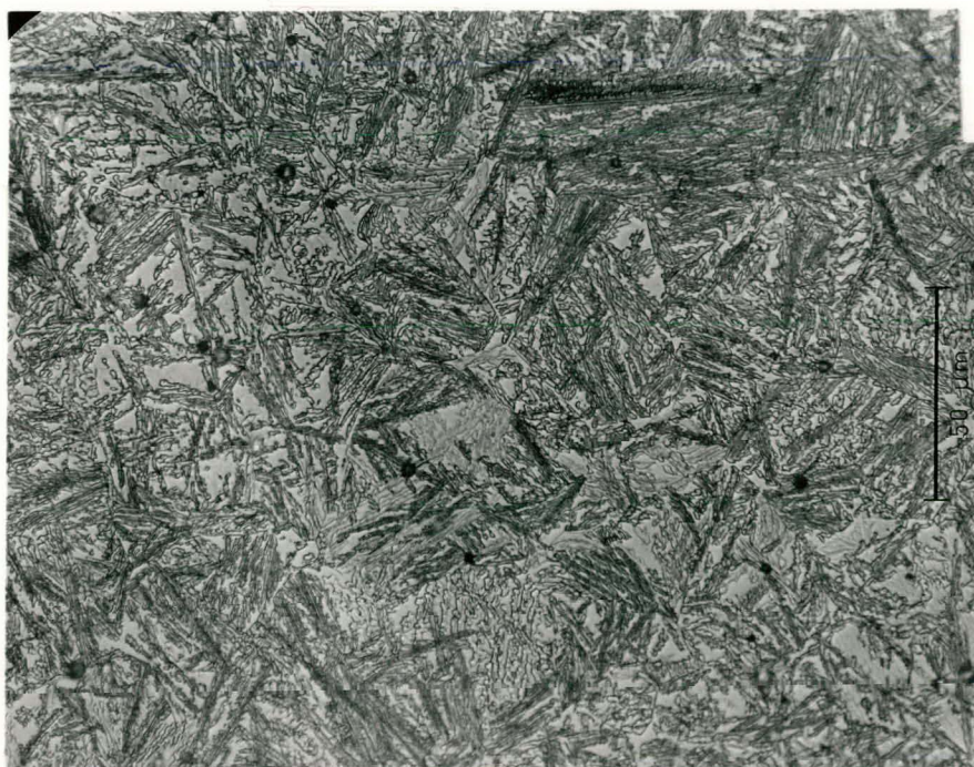
Figure 10. Optical micrographs of sample KHC18A austempered at 370° C for 5.5 hours (Nital etch) Magnifications: Top = 50X, Bottom = 500X
