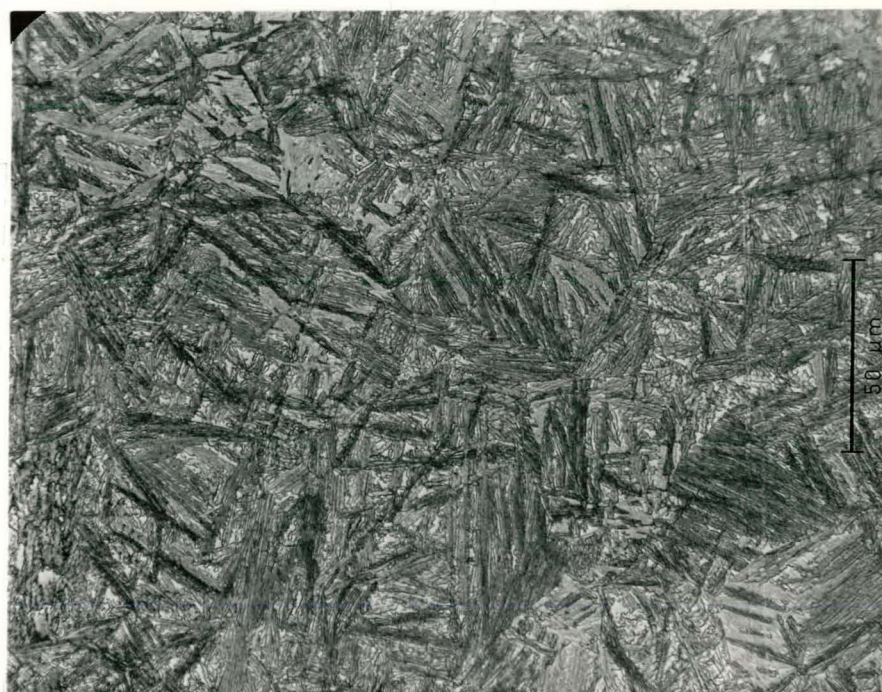
Figure 9. Optical micrographs of sample KHB16 austempered at 370° C for 5 hours (Nital etch) Magnifications: Top=100X, Bottom = 500X
