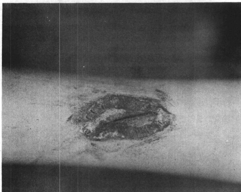
FIGURE 6. Photomicrograph of Deterioration of the Outer Layer of an 8YLY-S6 Glovebox Glove
