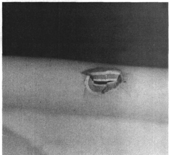
FIGURE 5. Photomicrograph of a Screwdriver-Blade Puncture of an 8YLY-S6 Glovebox Glove
