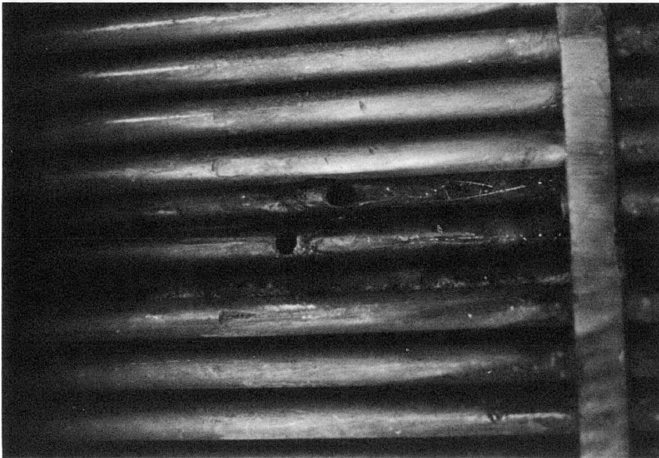
PHOTOGRAPH NO. 8 TUBE FAILURES DUE TO STEAM IMPINGMENT
