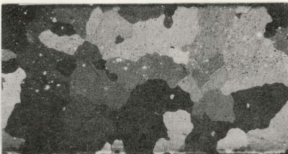
d. 1450°F/4 HRS 3.4% \epsilon_A 100% GRAIN COARSENING
