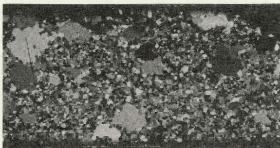
b. 1450°F/1 HR 3.4% \epsilon_A 23.7% GRAIN COARSENING
