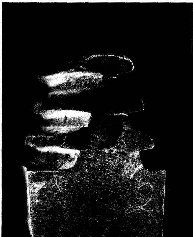
(a) Magnetic particle crack indications. Liquid fluorescent indicator.
