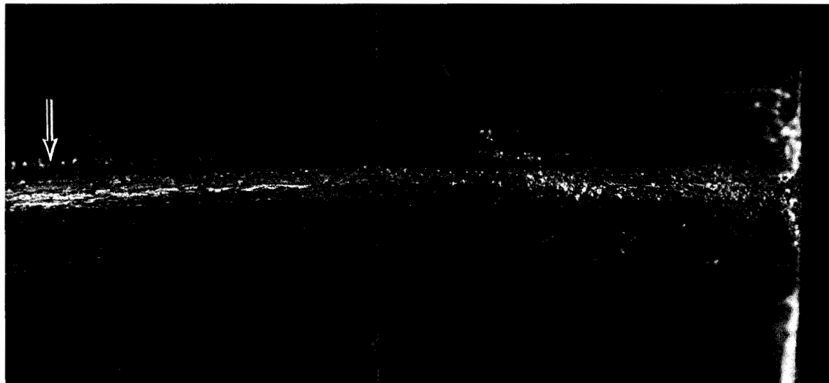
FIGURE 5-10. MAGNETIC PARTICLE CRACK INDICATION FOR CRACK 207-I-3bd, ROW 6R. Outlet face is at left. Arrows indicate match point. 4-1/2X
