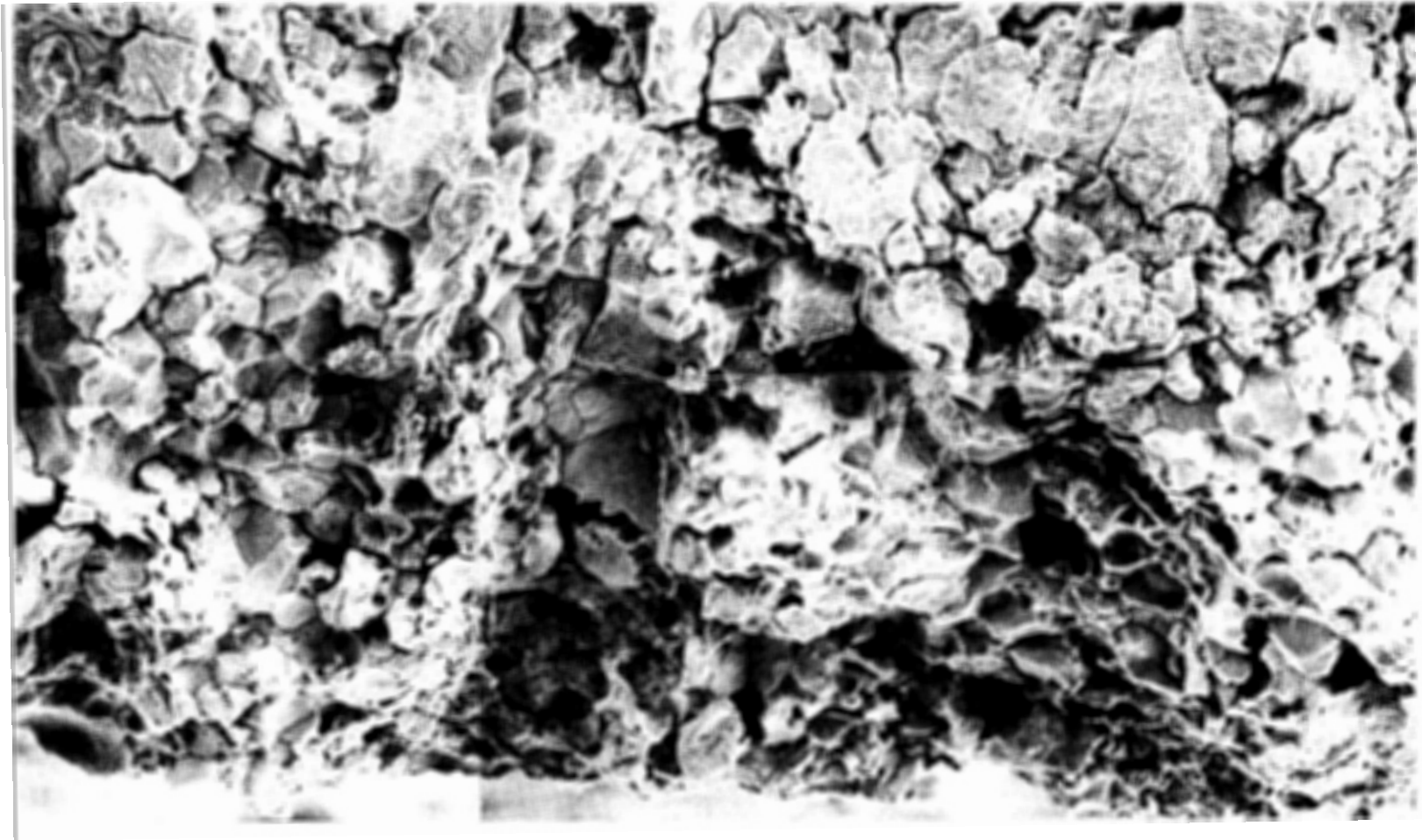
FIGURE E-4. TYPICAL TOPOGRAPHY OF CRACK 208-I-2b. Location 1, Figure E-3. SEM fractograph after cathodic cleaning. 200X
