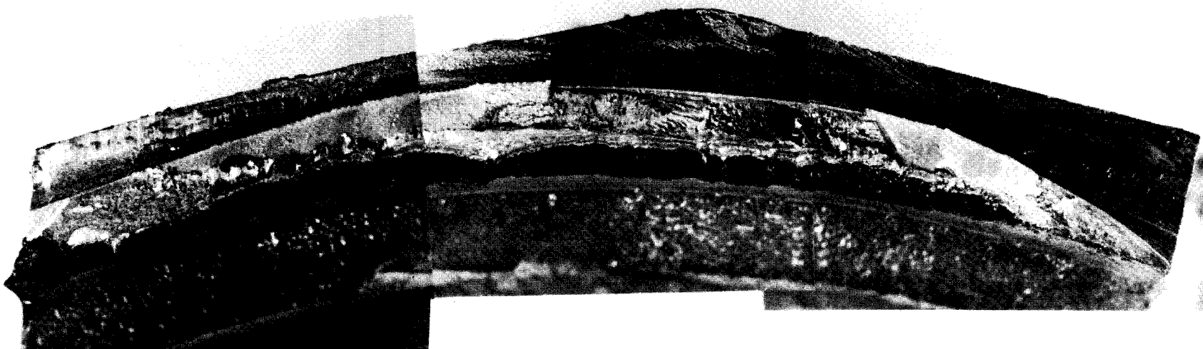
FIGURE 5-7. SURFACE OF CRACK 208-I-2bd, ROW 6R. View inward; outlet face is at left. See Figure 5-6. Fractographic features shown in Appendix E, Figures E-3, E-4 and E-5. 4X
