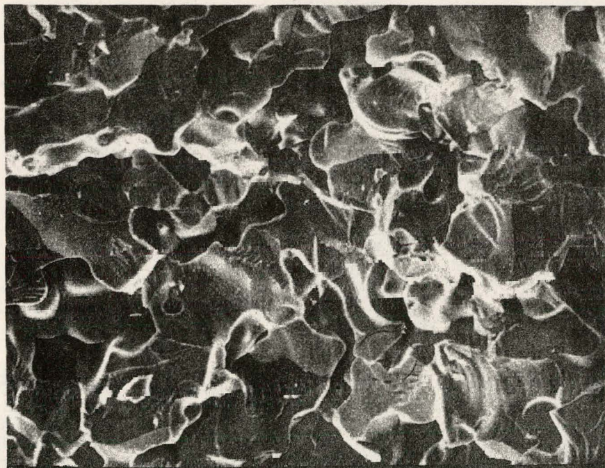
Figure 5.11 - Fractured surface of support tube, showing fused polycrystalline grains of calcia-stabilized zirconia (Sample 22B).
