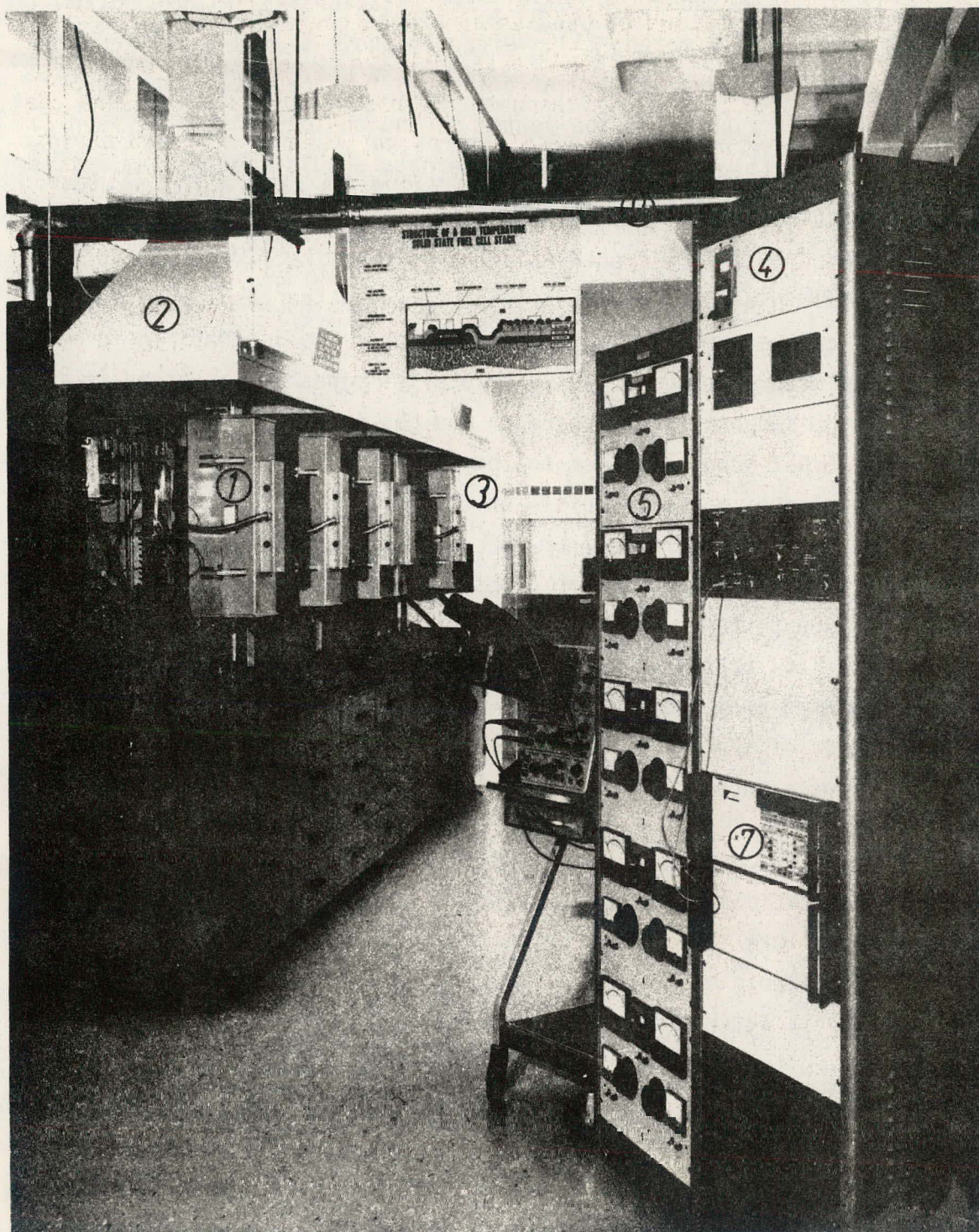
Fig. 5.21. General view of 5-station HTSOE fuel cell life test facility (left) and control and data acquisition system (right).
