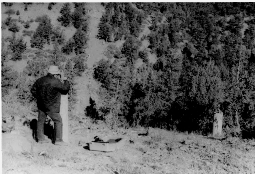
PHOTO 4 WILD T-2 THEODOLITE POSITIONED ON SURVEY MONUMENT
