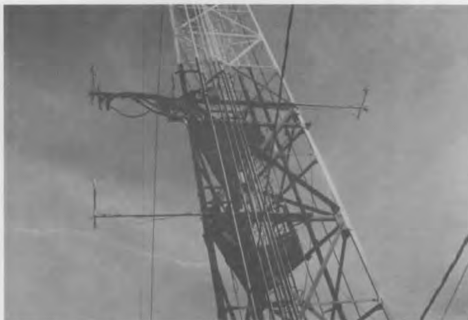
FIGURE 7. A Close-Up View of the Two Lower Monitoring Levels on the 410-ft Tower. The instrument booms at the 30- and 50-ft levels on the tower are visible. To gage the influence of the tower on the wind, measurements are made on two oppositely pointing booms at the 50-ft level.
