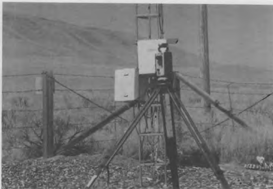
FIGURE 32. A View to the West-Northwest of the Base of the 30-ft Tower at the EOCC Monitoring Site. Rattlesnake Mountain is in the background. The surveying instrument in the foreground was used at each of the monitoring sites to determine their exact locations.
