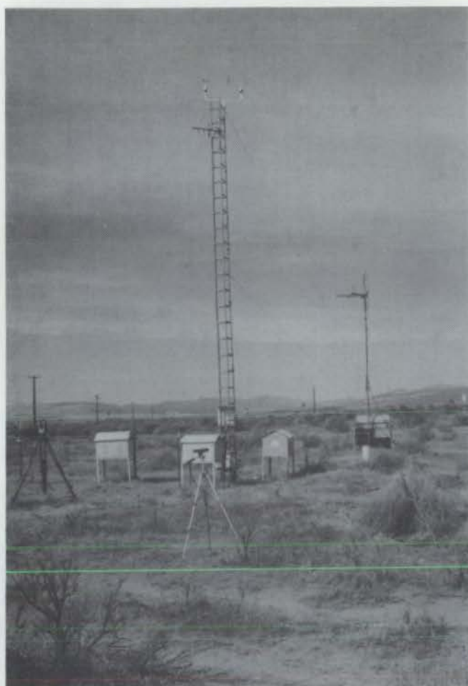
FIGURE 65. A View to the West of the 30-ft Tower at the YAKB Monitoring Site. Air sampling equipment is positioned around the base of the tower.
