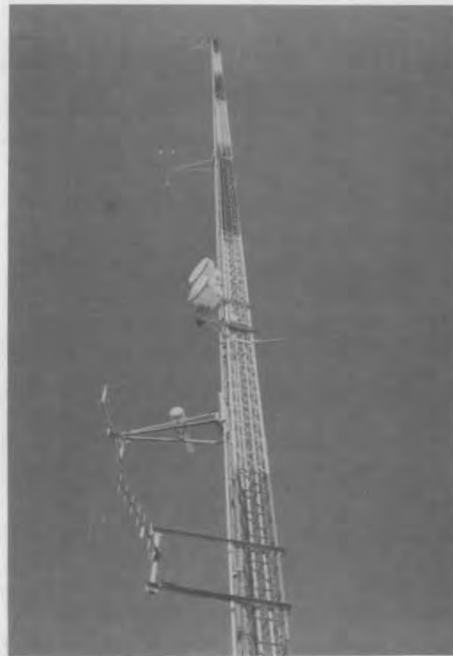
FIGURE 20. A Close-Up View of the 200-ft Tower at the 100N Monitoring Site. Instruments are mounted at the 30-, 100-, and 200-ft levels. Also on the tower are a UHF radio antenna and a microwave receiver/transmitter.
