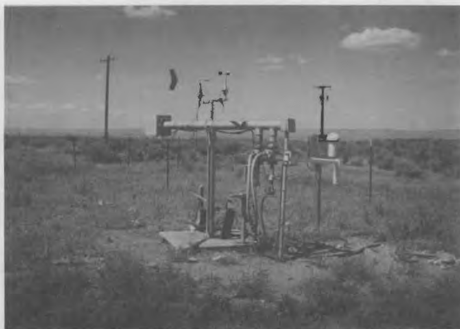
FIGURE 8. The Instrument Array Deployed 70 ft (25 m) North-Northwest of the Base of the 410-ft Tower. Wind sensors are deployed at 7 ft (2.1 m) above ground level, an air temperature sensor and a hygrometer at 5.5 ft (1.7 m) above ground level, and three sub-surface temperature sensors at varying depths in the sandy soil.
