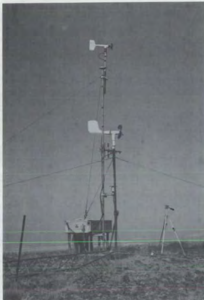
FIGURE 77. A Close-Up View to the Southwest of the Meteorological Instruments at the RMTN Monitoring Site. The site's wind sensors are mounted at the top of the taller pole. The larger wind instrument on the shorter pole provides data for the astronomical observatory and is not part of the site.
