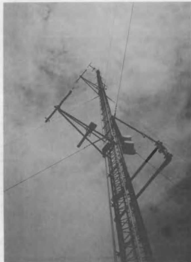
FIGURE 12. A Close-Up View of the 200-ft Tower at the 300A Monitoring Site. Instruments are mounted at the 30-, 100-, and 200-ft levels. Also on the tower are a UHF radio antenna and a microwave receiver/transmitter.
