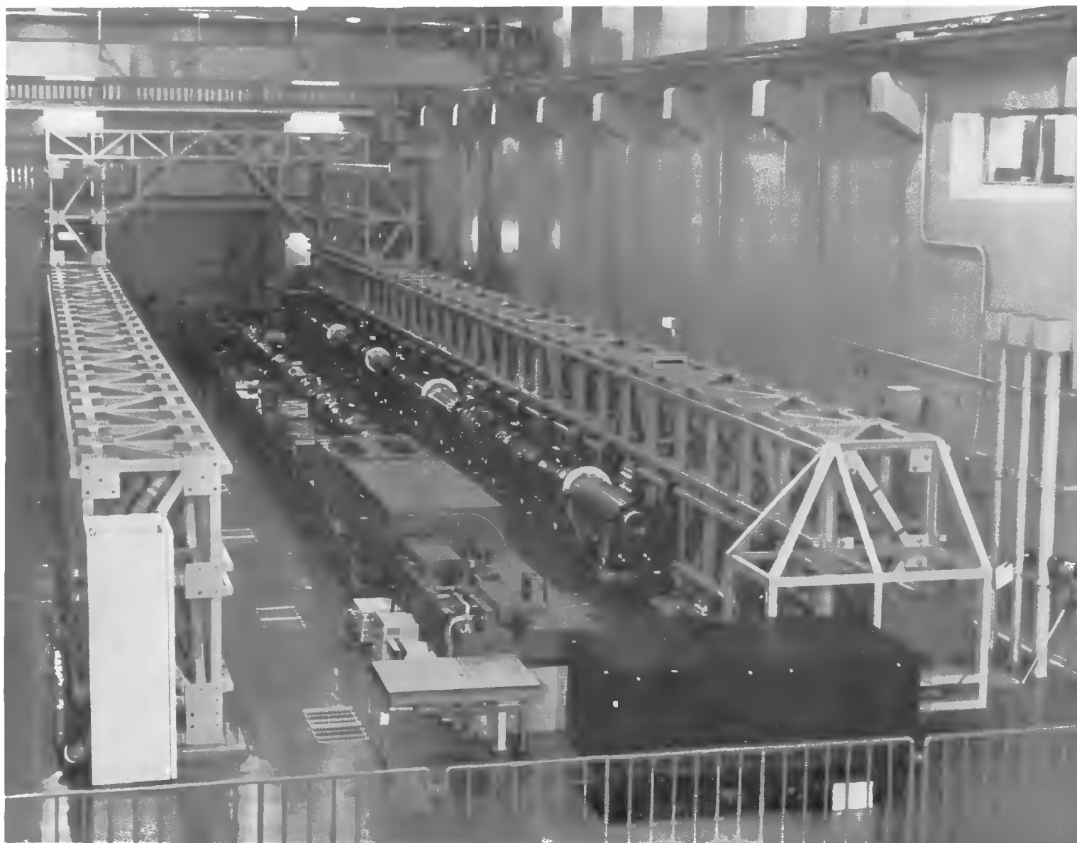
Fig. 2 — Recent picture of Gekko XII, showing the oscillator and preamplifier section in the center, and the first test arm on the right hand side.
