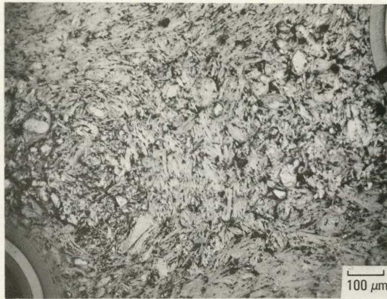
Fig. 5-43. Representative metallographic cross section of CERCA natural type matrix in CEA type e fuel rod. The rod was irradiated in capsule GF-1 (location 1-2) to a fast fluence of 5.5 \times 10^{25} n/m 2 ( E > 29 fJ) HTGR at 1080°C. A matrix microporosity of 13% was measured.
