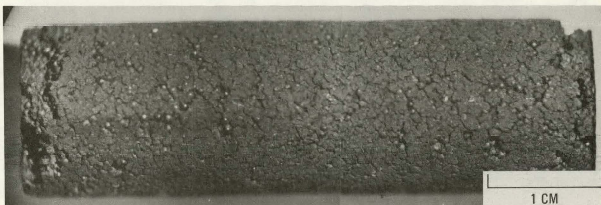
Fig. 5-8. Fuel rod compact No. 5 irradiated in GF-1 to 6.5 \times 10^{25} \text{ n/m}^2 ( E > 29 \text{ fJ} ) HTGR and at 1170^\circ\text{C} . This fuel rod is classified as type b [TRISO 500- \mu\text{m} -diameter (8Th,U) \text{O}_2 , 100- \mu\text{m} buffer/BISO ThO 2 ] and was fabricated by GA. (Two views at 180-deg rotation.)
