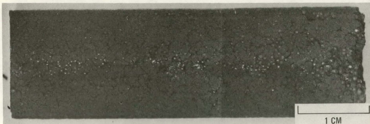
Fig. 5-9. Fuel rod compact No. 6 irradiated in GF-1 to 6.1 \times 10^{25} \text{ n/m}^2 ( E > 29 \text{ fJ} ) HTGR and at 1170^\circ\text{C} . This fuel rod is classified as type b' [TRISO 500- \mu\text{m} -diameter (8Th,U) \text{O}_2 , 80- \mu\text{m} buffer/BISO ThO 2 ] and was fabricated at GA. (Axial view shown.) Note localized chipping and fuel particle spalling.
