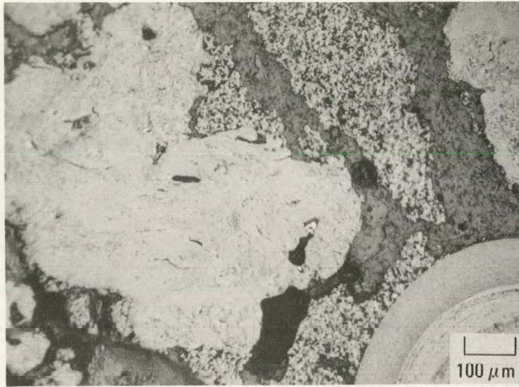
Fig. 5-41. Representative metallographic cross section of matrix and shim material in a GA type a fuel rod. The rod was irradiated in capsule GF-1 (location 2-4) to a fast fluence of 6.7 \times 10^{25} n/m 2 ( E > 29 fJ) HTGR at 1170°C. The matrix microporosity was not measured; however, it was estimated at ~50%.
