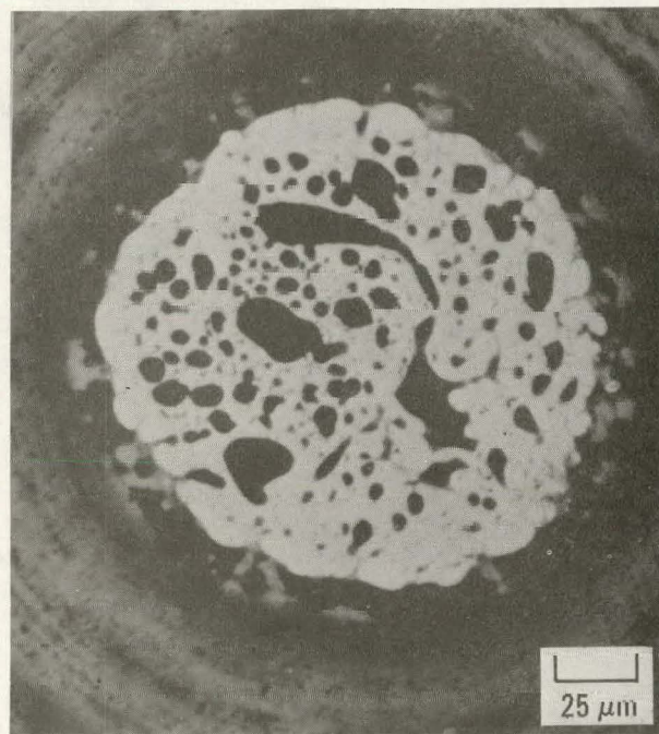
Fig. 5-61. Representative photomicrographs of unbonded TRISO UC 2 particles (6151-00-010) irradiated in capsule CF-1 (planchet 6) to a fast fluence of 2.7 \times 10^{25} n/m 2 ( E > 29 fJ) HTGR and a burnup of 50% FIMA at 1095°C
