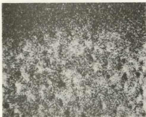
Fig. 5-91. Back-scattering electron image defining C, Al, Si, Cs, and Ba distributions in BISO-coated (8Th,U)O 2 , batch 611-105E irradiated in GF-3 to a fast fluence of 9.0 \times 10^{25} \text{ n/m}^2 ( E > 29 \text{ fJ} ) HTGR and 11% FIMA at 1000°C. These kernels were doped with 2 Al + 2 Si.
