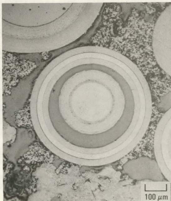
Fig. 5-56. Representative photomicrographs of TRISO inert particles (6351-01-020) from type b' fuel rod (7161-003-03-5) irradiated in capsule GF-1 (location 3-6) to a fast fluence of 6.1 \times 10^{25} \text{ n/m}^2 ( E > 29 \text{ fJ} ) HTGR and a burnup of 9.4% FIMA at 1170°C
