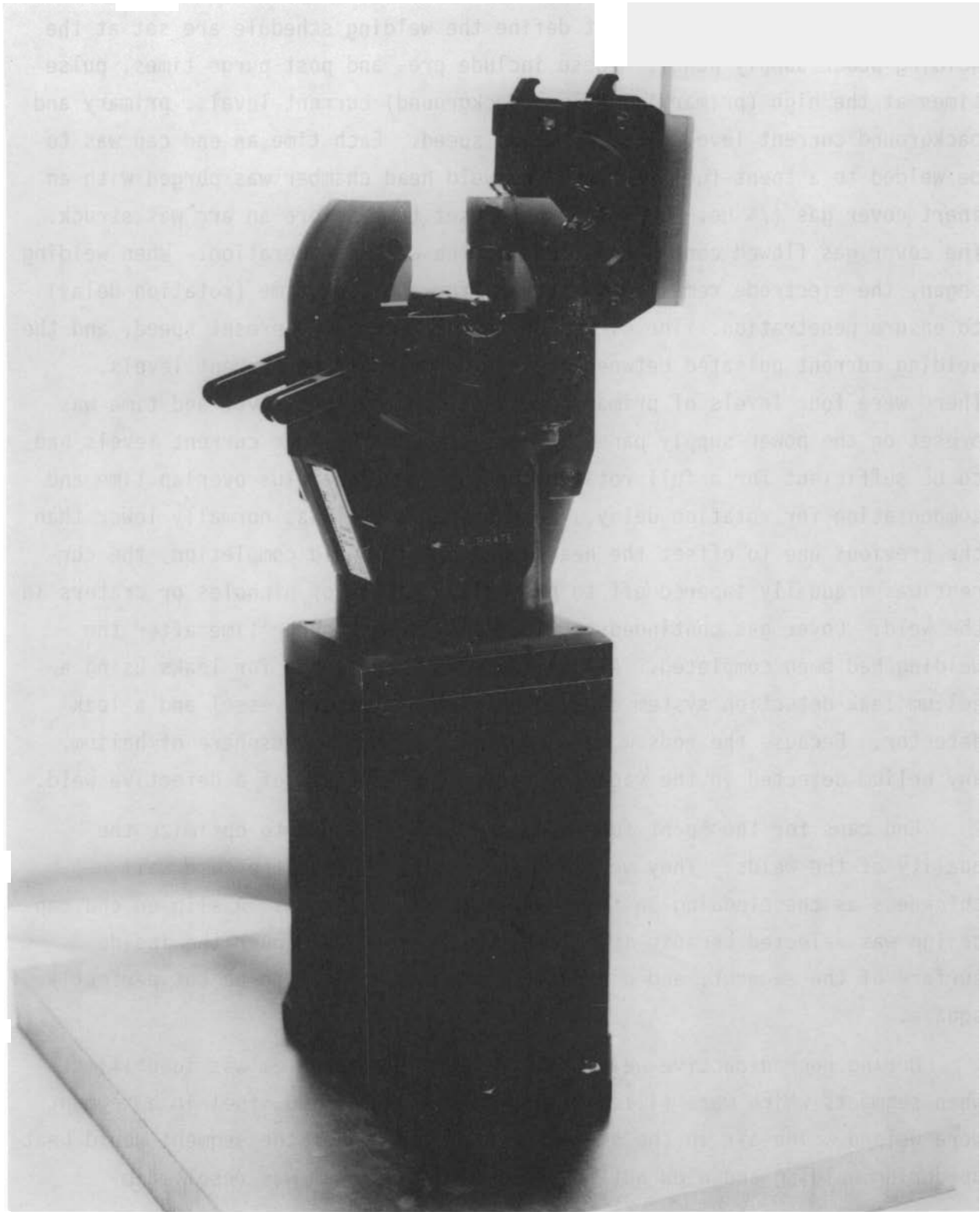
FIGURE 7. Spent-Fuel-Rod Segment TIG Orbital Head Welder
