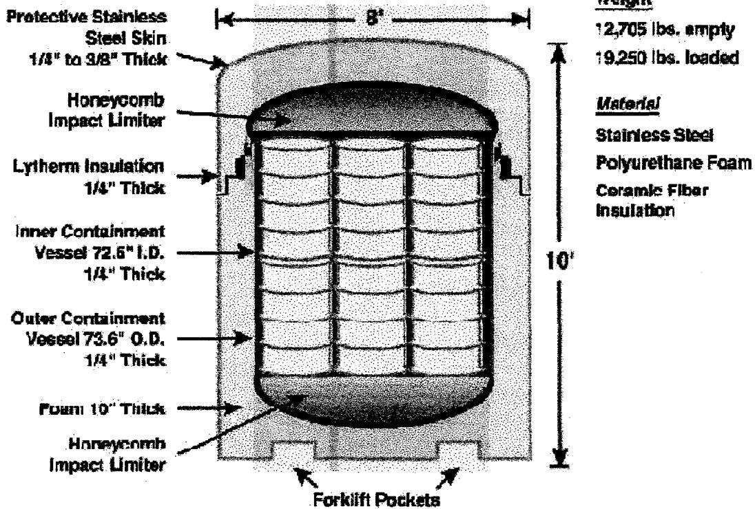
The TRUPACT-II has been certified to transport TRU waste to WIPP. The certification process includes stringent package testing.
