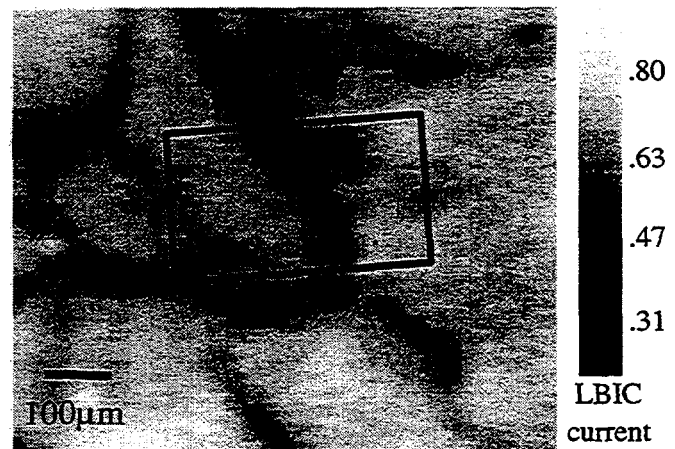
Figure 1: Light Beam Induced Current map of carrier recombination across a portion of multicrystalline silicon. Dark regions indicate high carrier recombination. The black box denotes the area analyzed with x-ray fluorescence.
